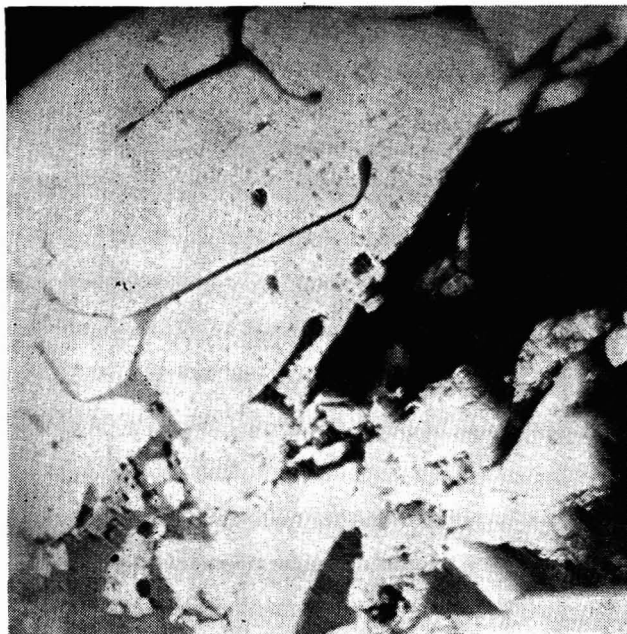
Figure 4. Photomicrograph of Ammonia Synthesis Catalyst Showing Mosaiclike Structure
