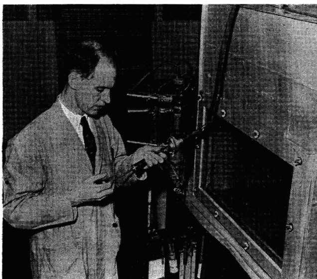
Figure 2. Calibrating Paper with Known Quantities of Hydrofluoric Acid
