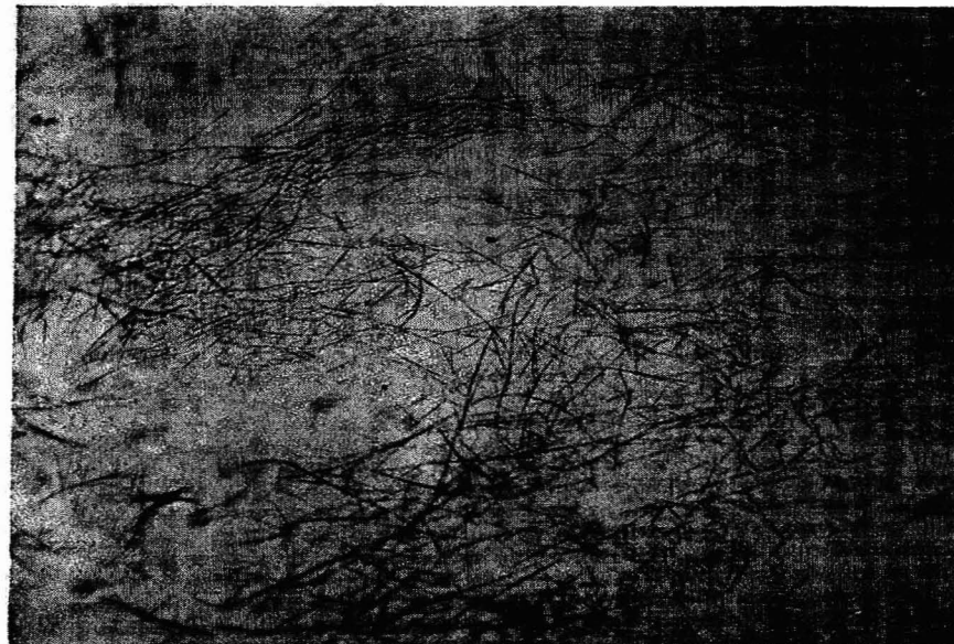
Figure 1. Nickel Compound of 1,2-Cyclohexanedione Dioxime Precipitated from Pure Nickel Sulfate Solution ( \times 258 )
