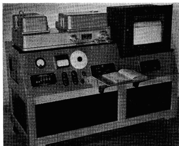
Figure 2. Mobile Spectrometer Unit Showing Detachable Notebook Shelf in Place
