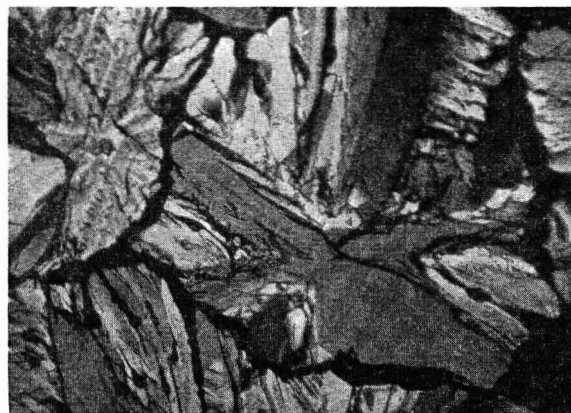
Figure 17. 95% Alpha Fusion (Crossed Nicols) Showing Smaller and More Irregularly Shaped Spherulites
