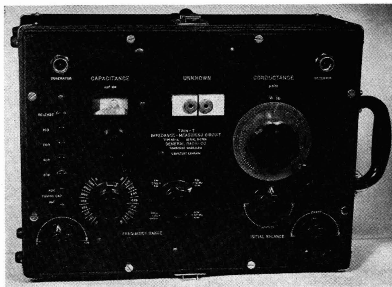
Figure 3. General Radio Twin-T Impedance-Measuring Circuit
