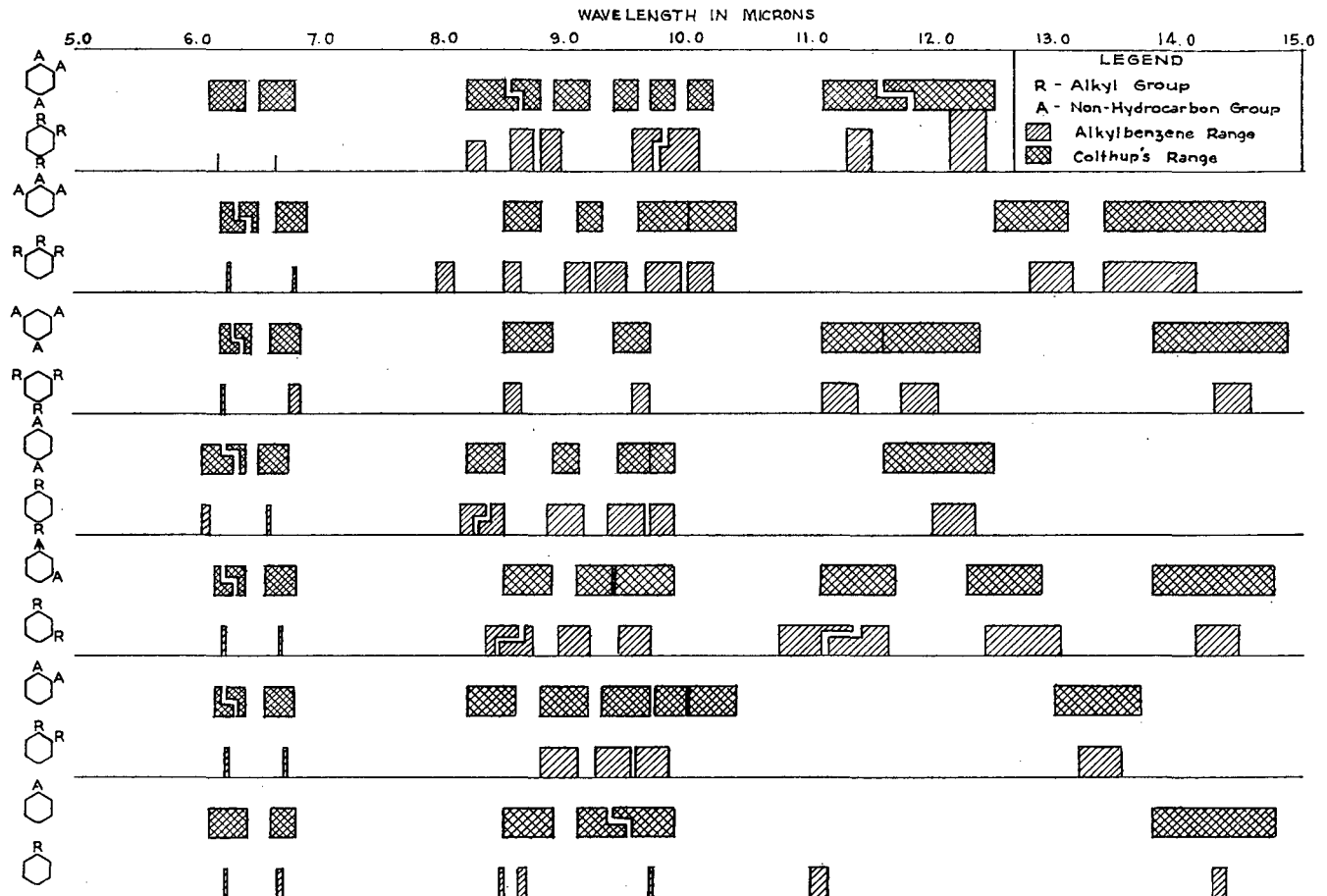
Figure 8. Comparison of Correlations Determined from Alkylbenzene Spectra Only and All Substituted Benzene Spectra
