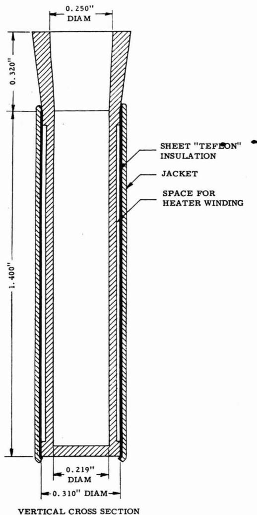
Figure 4. Diagram of 0.5-Ml. Calorimeter
