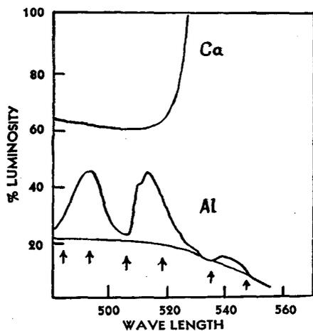
Figure 3. Emission Spectrum of Calcium and Aluminum
