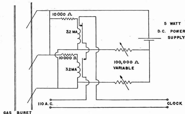
Figure 3. Stop-Clock Starting and Stopping Circuit
