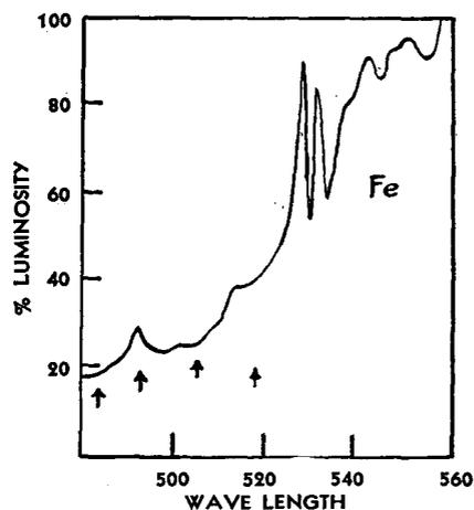
Figure 4. Emission Spectrum of Iron
