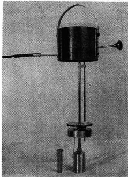
Figure 6. Inner Assembly of Radiation Shield with Calorimeters
