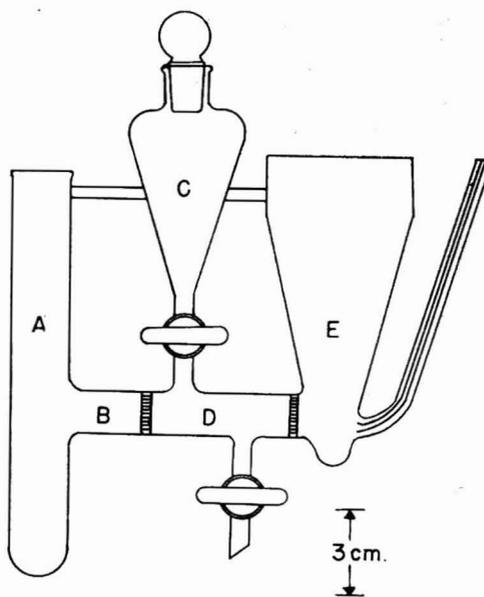
A cell of rugged construction has been designed to eliminate these problems. Volumes of solution from 2 to 55 ml. may be analyzed, and the opening is large enough so that a glass electrode may be permanently mounted in the stopper, if desirable.
