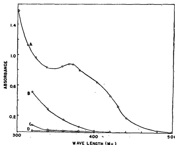
Figure 2. Absorption Spectra of Metal Diethyldithiocarbamates
