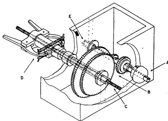
Figure 2. Transmission and Clutch Assembly for Variable pH Titration
