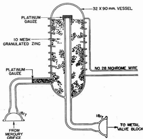
Figure 1. Diagram of Trap
