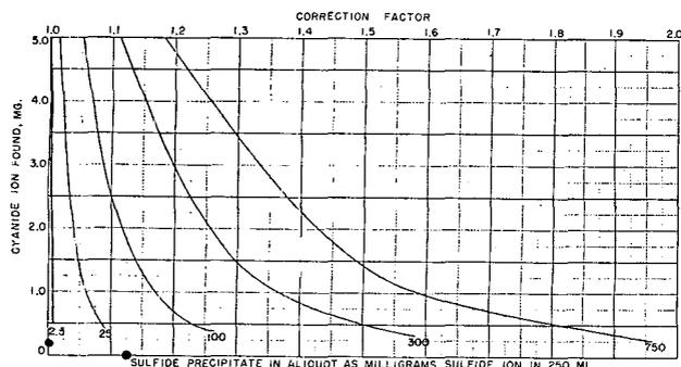
Figure 1. Cyanide Ion Correction Graph
