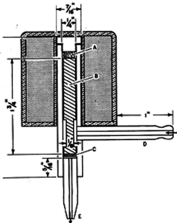
The valve chamber consists of a polystyrene barrel fitted into the plunger well of a Guardian Type No. 4-AC 115-volt alternating current solenoid. A polystyrene side-arm inlet tube,  $\frac{1}{4}$  inch in outside diameter,  $\frac{1}{32}$  inch in inside diameter, is cemented to the plunger barrel. The outlet tube,  $E$ ,  $\frac{1}{4}$  inch in outside diameter has a bore of  $\frac{1}{4}$  inch. The valve seat of the outlet tube is smoothly turned on a lathe to ensure a flat seat.
