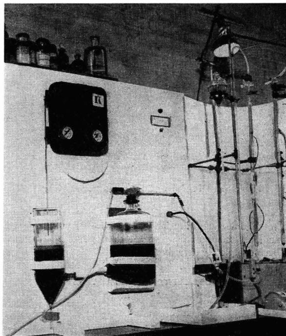
Figure 7. Pressure Control System
