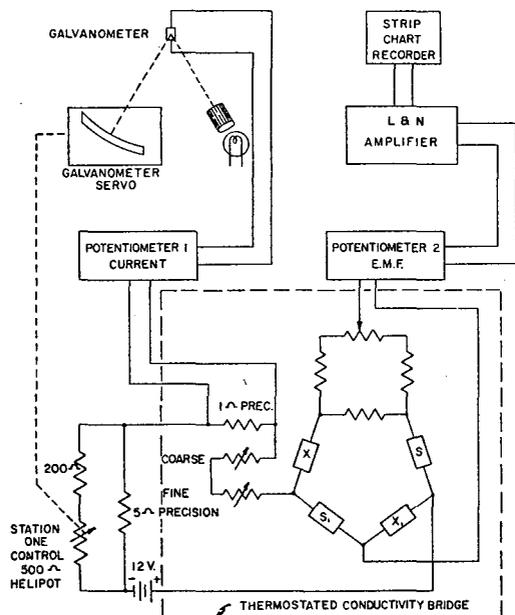
**Figure 1. Schematic Diagram of Current Control for Gas Analysis Apparatus**
