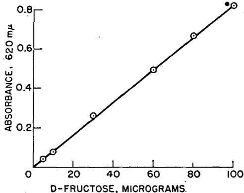
**Figure 1. Absorbance Curve, Alcoholic Anthrone Method**
