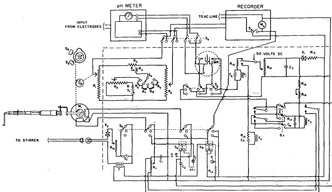
Figure 4. Circuit Diagram of Assembly for Constant pH Titration
