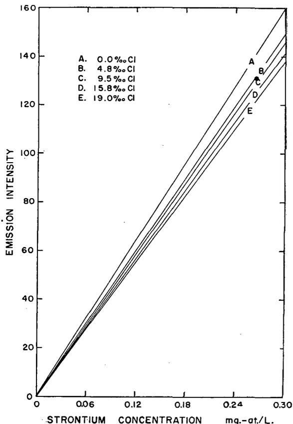
**Figure 1. Calibration Graphs of Strontium in Synthetic Sea Water**
