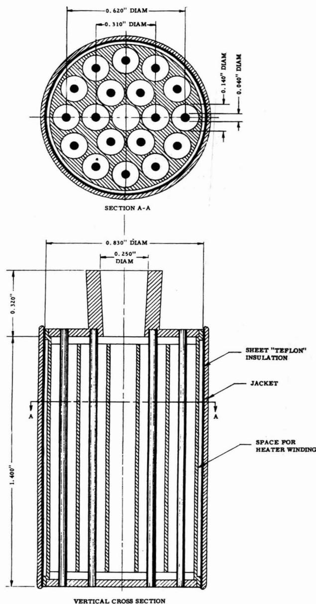
Figure 3. Diagram of 5-Ml. Calorimeter
