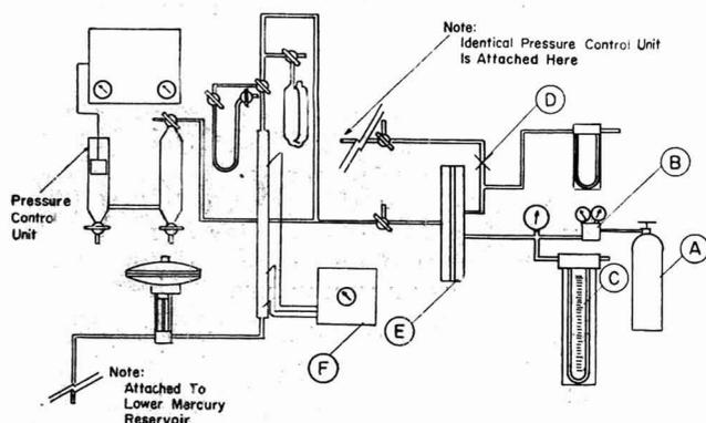
Figure 2. Diagram of Automatic Gas Buret Separation Apparatus
