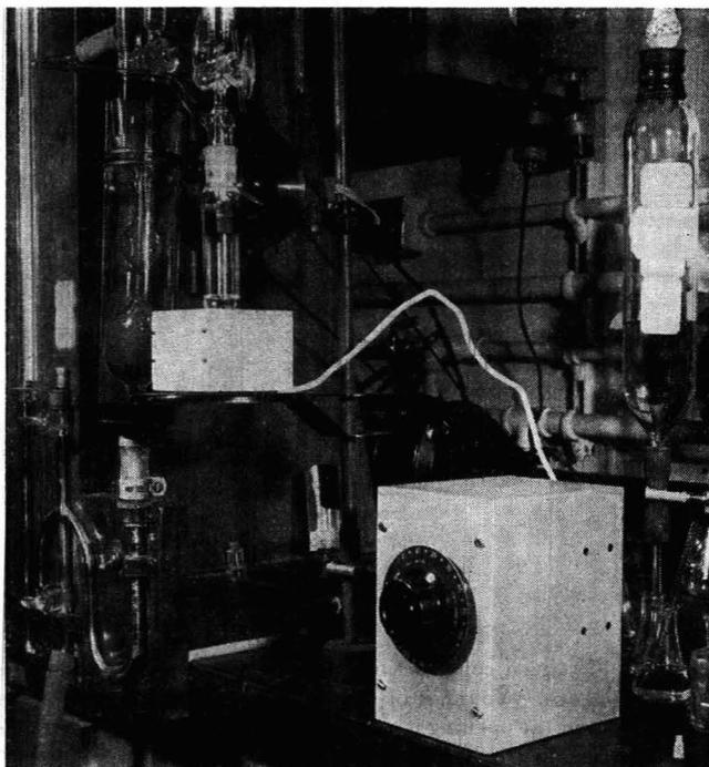
Figure 1. Heater Assembly with Resistance Assembled with Van Slyke Combustion Equipment
