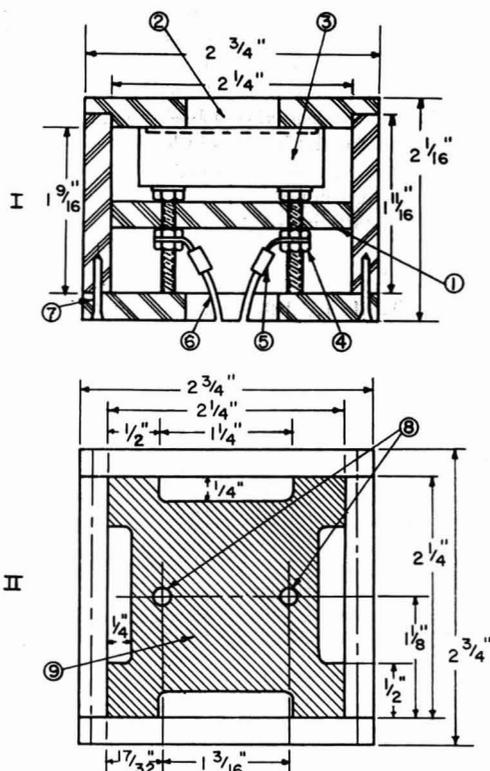
Figure 3. Scale Drawings of Heater Unit Assembly
