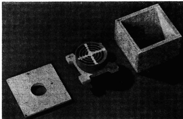
Figure 2. Separated Parts of Heater Assembly
