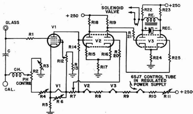
Figure 2. Schematic Diagram of pH-Sensitive Electrical Controller
