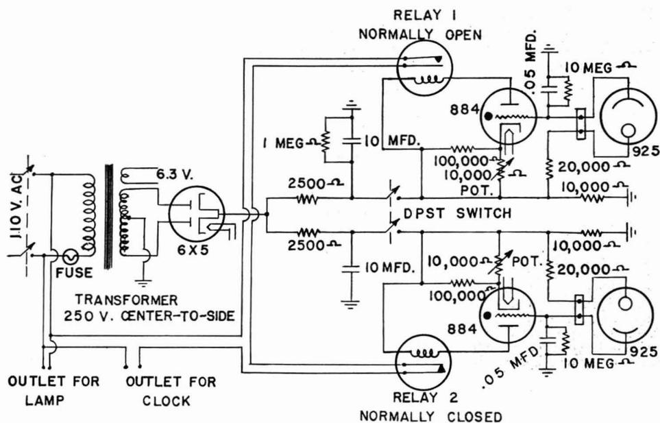
Figure 5. Diagram of Photoelectric Relay
