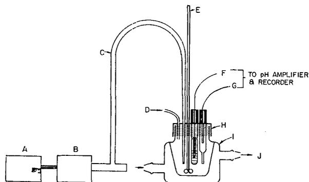
Figure 1. Cell and Experimental Arrangement for Variable pH Titration
