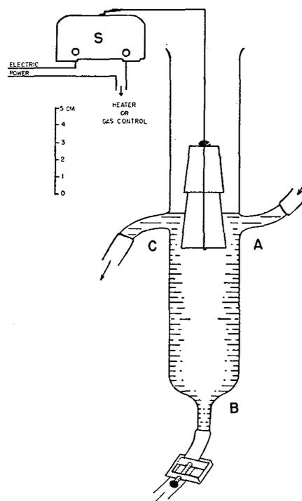
the remainder of the system. Safety devices described include a thermoregulator sealed into the system for protection of electrically heated water stills (3), a pressure-sensitive relay (1), and more recently, a bellows-type pressure switch (2) for use in conjunction with a mercury diffusion pump or other electrically heated equipment. The device described here is of simple construction and has been in use for some time with a mercury diffusion pump.
