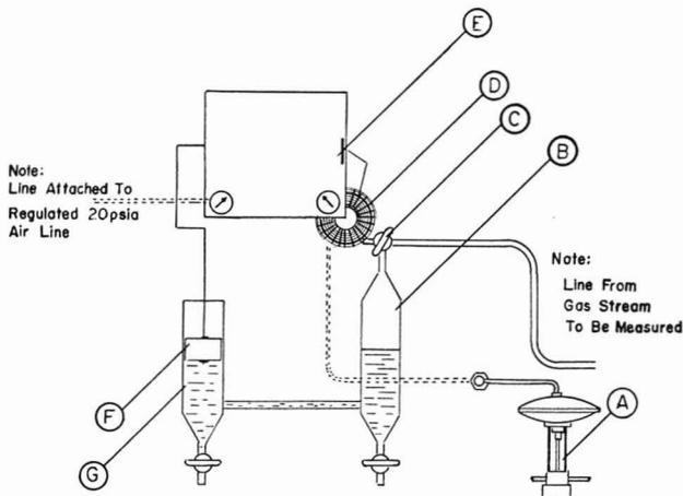
Figure 6. Diagram of Pressure Control System
