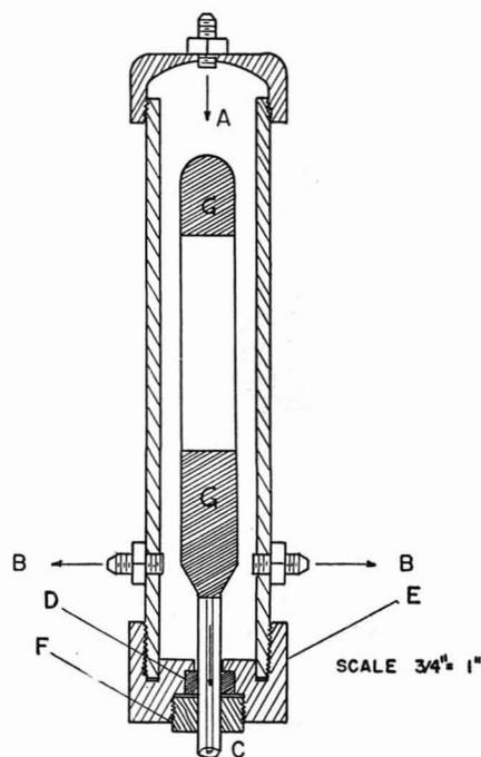
Figure 9. Thimble Type of Diffusion Cell
