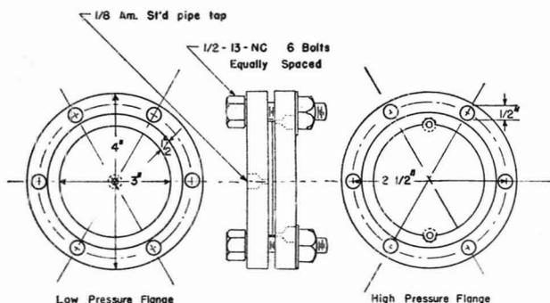
Figure 8. Diagram of Flanged Separation Cell
