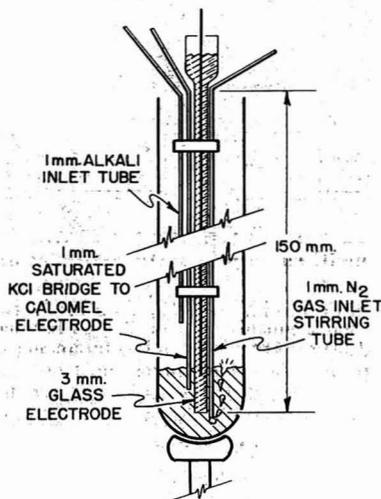
Figure 3. Glass-Calomel Electrode Assembly
