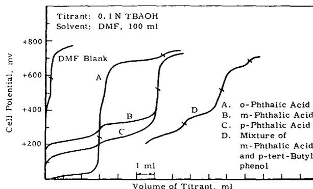
**Figure 9. Phthalic Acid Isomers Titrated in Dimethyl Formamide**
