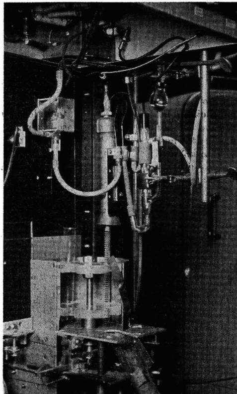
Figure 6. Sample Changer Turnstile Mechanism
