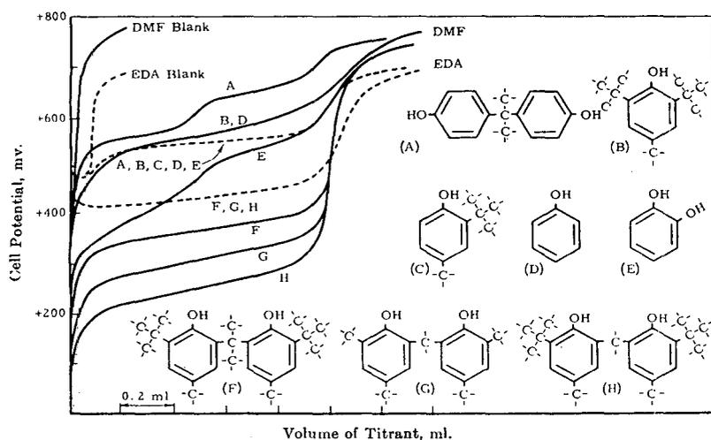
**Figure 6. Phenolic Compounds Titrated in Ethylenediamine and Dimethyl Formamide**
