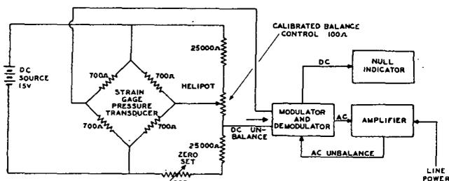
Figure 3. Simplified Diagram of Reid Vapor Pressure Indicator
