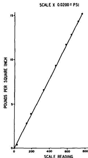
Figure 4. Calibration of Reid Vapor Pressure Apparatus
