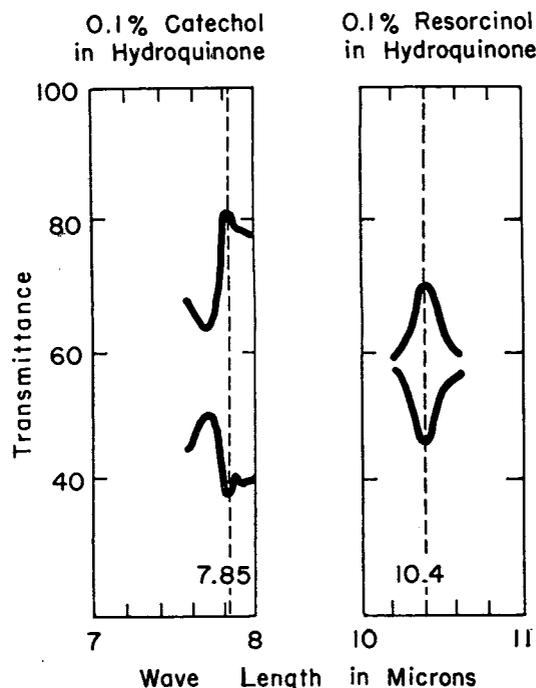
**Figure 2. Typical Absorption Curves**
