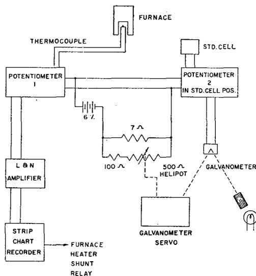
Figure 3. Schematic Diagram of Voltage-Controlling System
