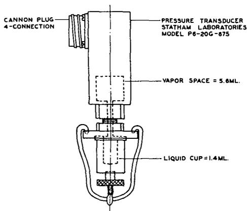
Figure 2. Pressure Transducer and Cell Assembly
