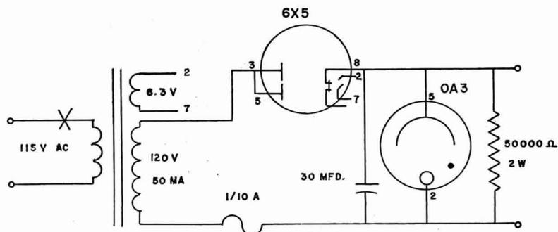
Figure 4. Five-Watt Direct Current Power Supply
