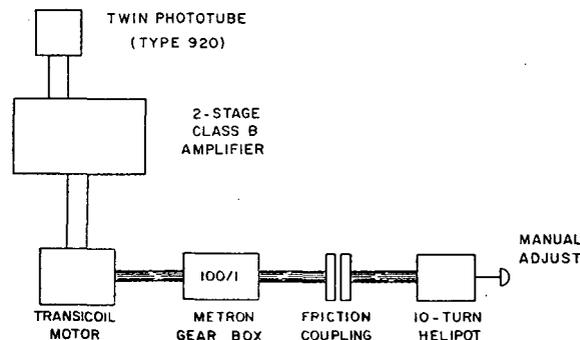
**Figure 2. Block Diagram of Galvanometer Servo**
