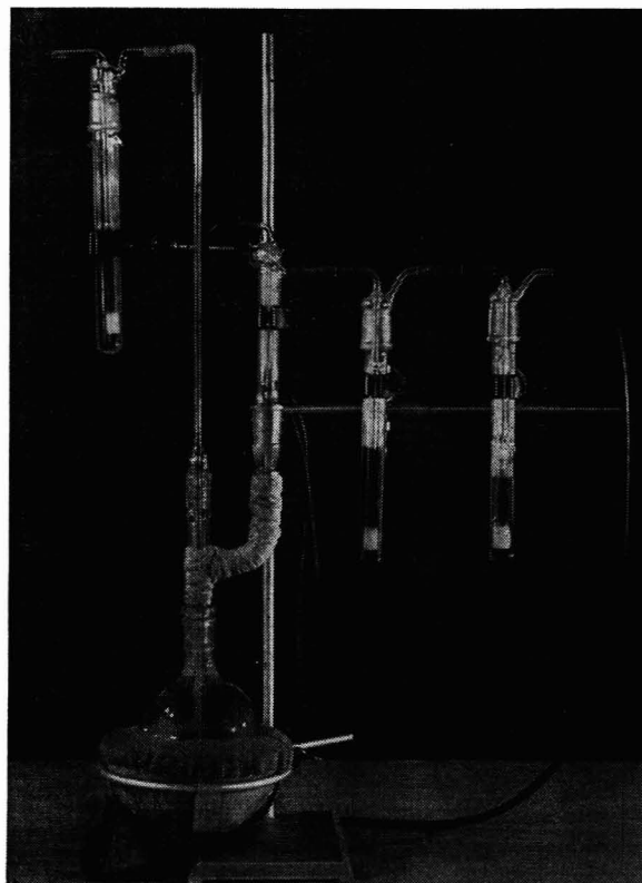
Figure 1. Apparatus for extractive decomposition of rubber compounding materials
