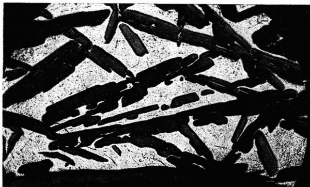
Figure 3. Micrograph of top section of iron ingot held in a graphite crucible
