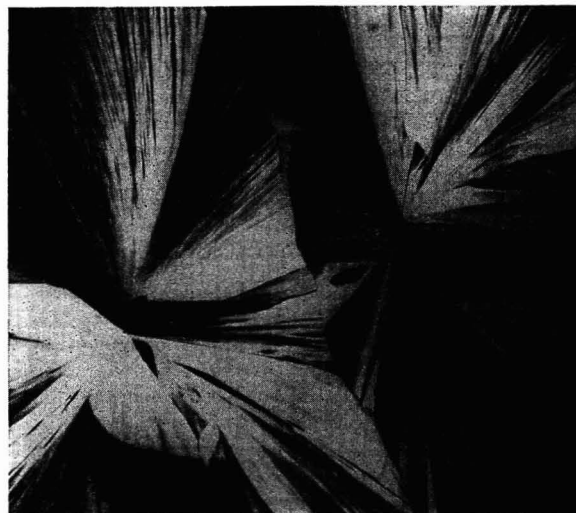
Figure 3. Crystals of decomposition product obtained on melting or subliming 4-aminosalicylic acid
