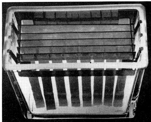
Figure 2. Arrangement of stainless steel rack and one row of filter paper strips
