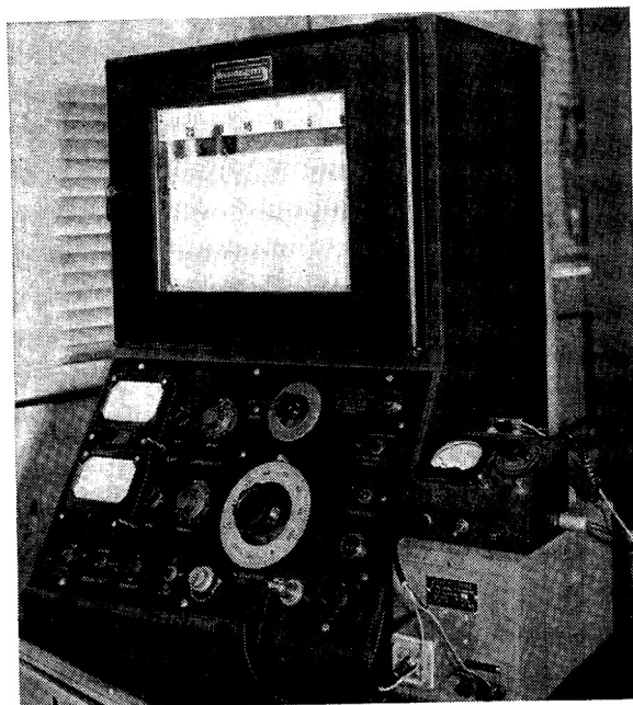
Figure 2. Typical setup of compensator, using commercially available amplifier
