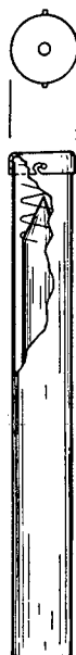
Figure 2. Steel casing and cover containing sealed tube to be placed in rocking furnace
