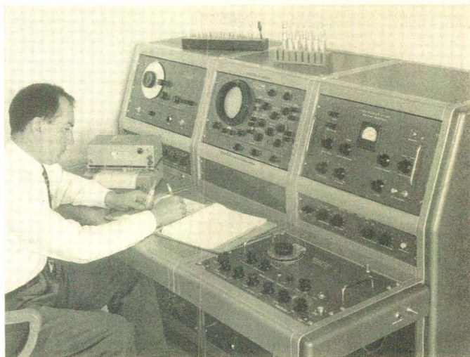
Varian Model V-4300-2 Dual Purpose N-M-R Spectrometer console. Not shown: associated Super High Resolution 12-inch Magnet System.
