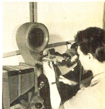
The Balphot metallograph is used in many metallurgical studies of semiconductor materials. Here, the p-n junction of a large silicon diode is being examined. This laboratory also includes equipment for sample preparation, microphotography, and melting point determination of alloys
