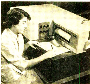
OPERATOR RUNNING CURVE of a color sample on the General Electric's easy-to-use Recording Spectrophotometer.
