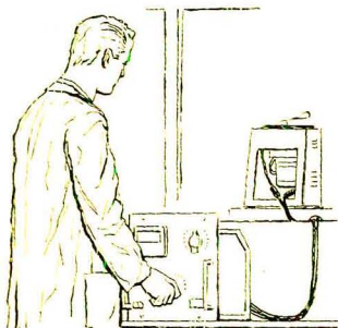
Centrifuge Inside — Controls Outside the Cold Room or Chamber
