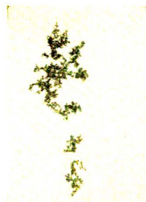
Electron Micrograph of sludge particles in diesel fuel oil. Oil treatment has been improved considerably by new information obtained on the character of sludge-forming materials.
