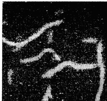
Figure 3. Scan over cast iron sample with carbon K\alpha radiation detection
