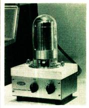
Calorimeter cell shown is the latest plug-in accessory for the Model 900 differential thermal analyzer. The cell measures specific heat and determines heats of transition and reaction in the range from  $-100^{\circ}$  to  $700^{\circ}$  C. Thermal data obtained with the cell supplements information provided by the basic Model 900 DTA unit. E. I. du Pont de Nemours & Co., Wilmington, Del.
