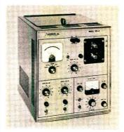
Model 15C Series, designed for both modular and integrated construction concepts, provides the choice of over 2000 feature combinations for gas chromatography. The instrument can be single or dual column, isothermal or temperature programmed. Multiple column switching systems and a choice of all types of detector systems plus two different oven arrangements are possible. Loenco, Inc., 2092 N. Lincoln Ave., Altadena, Calif. 425
