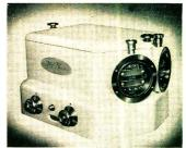
Model 218, 0.3 meter plane grating scanning monochromator, operates in the range 1050 A. to 16 microns. First order resolution is better than 0.25 A. The instrument features special aspheric optical surfaces and snap-in type gratings. Conversion from atmospheric to vacuum operation and flexibility of positioning are offered. McPherson Instrument Corp., 530 Main St., Acton. Mass. 01720. 420
