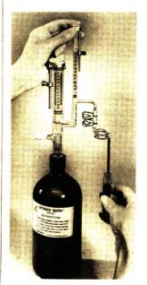
... your procedures with all-PYREX L/I RE-PIPETS\* and Automatic Dilutors\*. Using your reagents and your bottles, complete your procedures in 1/10 the time with far greater accuracy—and without cleanup. Absolute accuracy 1%, reproducibility  $\pm 0.1\%$ . Just press a plunger to dispense, dilute, transfer and mix volumes from microliters to deciliters.
