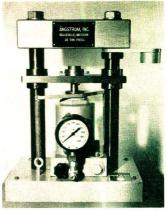
Briquetting press, Model 4500 for routine preparation of x-ray, optical emission, and infrared samples, is a 30-ton press with a two-stage pump for rapid operation. A swing-away anvil allows easy die access. Briquets are formed in one simple operation and there is no need to remove the die to eject the specimen. Standard molds from ½" to 1¾" in diameter are used. Angstrom, Inc., 2454 West 38th St., Chicago 2, III.
