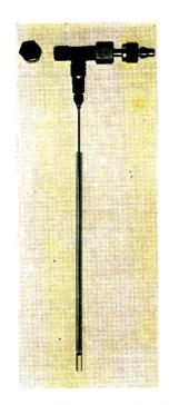
Figure 1. NMR microtube with 17gauge syringe needle and 1/4-inch tubing T
