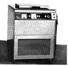
Model 806 C5 Size 2 - refrigerated economy centrifuge. Operating speeds from 2,500 rpm. Temperature range from  $+5^{\circ}$ to  $+30^{\circ}$  C. with fixed heads and 25° C. ambient temperature.  $+15^{\circ}$  to  $+30^{\circ}$  C. with trunnion heads. Specify whether 208v or 230v if desired. \$1995.00
