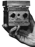
SMALL... BUT MIGHTY — This "mini" stir plate is compact and light. Total weight is only 2-1/2 lbs. The sturdy cast aluminum top is 3-5/8" square. Dovetail bracket provided for rack set-ups.
