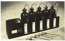
Now anyone can get accurate, reliable biochemical oxygen demand water quality determinations without complicated procedures, calculations or previous training. Hach Model 2173 manometric BOD measurements compare within ±5% of standard APHA dilution procedures and, at the same time, cost less to operate than other manometric set-ups used (Warburg and Sierp).
