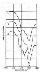
Figure 5. Infrared spectra of molecular distillation fraction from Wilmington asphalt in carbon tetrachloride (I), methylene chloride (II), and tetrahydrofuran (III)
