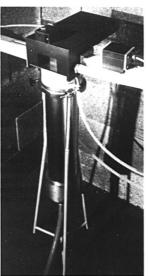
This density is sufficiently high to overcome the low reaction cross sections of many materials and the generator is thus ideal for a wide variety of industrial and laboratory analytical applications.
