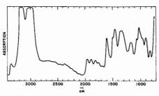
Figure 5. Spectrum of polystyrene (5-sec scan)
