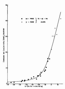
Figure 5. Plot of phase-insensitive corrosion maxima in 10% (COOK), solution  $vs.\ b$  equal to a linear function of the manganese and aluminum content of the corresponding alloys
