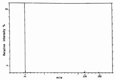
Figure 5. Normalized mass spectrum of nortriptyline. Molecular ion = 263 with a relative intensity of 0.4%
