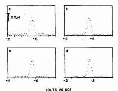
Figure 8. Derivative pulse polarograms of  $4 \times 10^{-5} M$  Cd<sup>1+</sup>, 0.5 M KNO<sub>1</sub>
