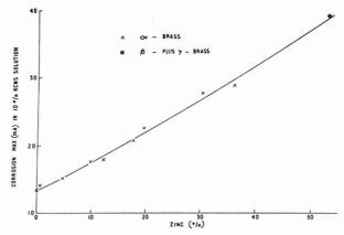
Figure 6. Plot of phase-insensitive corrosion maximum in 10% KCNS solution vs. zinc content for a number of brasses
