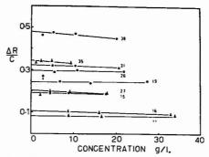
Figure 5. Effect of asphalt fraction concentration in VPO method for measuring molecular weight
