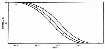
Figure 1. Equilibrium concentration of the TIDDTC in the chloroform phase as the function of EDTA concentration at different pH values
