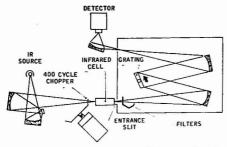
Figure 1. IR-GC spectrometer optical system layout
