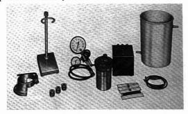
You can rely on sulfur values as determined by the PARR bomb combustion method using ASTM D129, D271 and related standard techniques.
