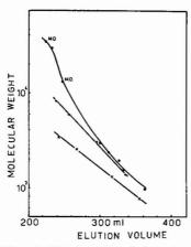
Figure 4. Molecular weights of selected fractions from the asphaltenes in different solvents
