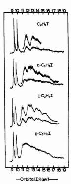
Figure 4. Photoelectron spectra of some aliphatic iodo compounds, excited by irradiation with 584-Å photons
