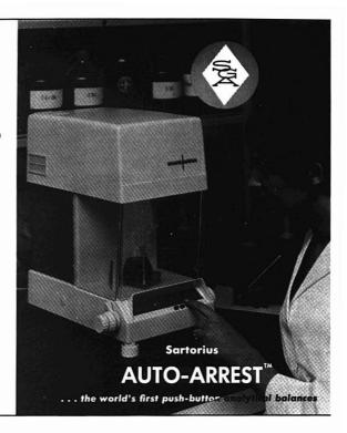
Three new balances have been added to the popular Sartorius Series 2400 line; however, in place of a lever, you arrest and release Models 2472, 2474 and 2492 by pushing a button. This causes a small motor to activate the arrestment system, guaranteeing the smoothest possible weighing technique. Since accidental "jarring" can't occur, chipped knife edges are impossible.
