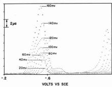
Figure 5. Derivative pulse polarograms of  $4 \times 10^{-5} M \text{ Cd}^{2+}$ , 0.5  $M \times NO$ ,
