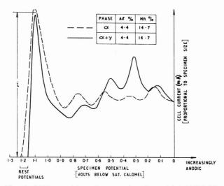
Figure 2. Initial range of the anodic current-voltage characteristic in  $30\,\%$  NaOH for two alloys of the same chemical composition but different phase constitution
