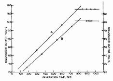
Figure 4. Pressuremetric titration curves of ammonium ion with electrogenerated hypobromite
