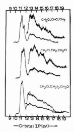
Figure 6. Photoelectron spectra of 1,2- and 1,3-dichloropropane and 1,4-dichlorobutane, excited by irradiation with 584-A photons
