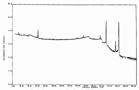
Figure 3. Gamma-ray spectrum of the Allende chondrite plus a ωCo source ωCo activity is 8.3 times the activity measured in the spectrum in Figure 2
