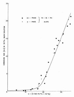
Figure 4. Plot of phase-insensitive corrosion maxima in 30 % NaOH solution  $vs.\ a$  equal to a linear function of the manganese and aluminum content of the corresponding alloys
