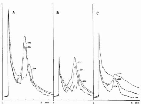
Figure 4. Base peak fragmentograms of 100 picograms (A) and 50 picograms (B) of NT-TFA, M-232, deuterated NT-TFA, M 234,
