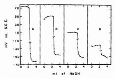
Figure 12. Titrations of 25 ml of 0.01 M HNO<sub>2</sub> with NaOH in the presence of varying concentrations of KNO<sub>2</sub>
