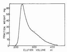
Figure 2. Weight distribution of fractions separated from the asphaltenes by GPC
