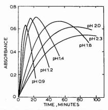
Figure 2. Effect of pH on time course of  $\alpha\text{-benzamido-benzylpenicillenic acid in presence of mercuric chloride at 50 °C in 19 % aqueous ethanol$
