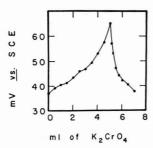
Figure 5. Titration of 50 ml of 0.01M BaCl<sub>2</sub> with K<sub>2</sub>CrO<sub>4</sub>
