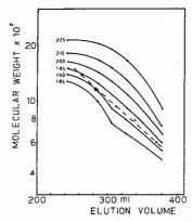
Figure 6. Best X ratio for coincidence of unit sheet weight with molecular weight for the asphalt fractions
