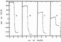
Figure 13. Titrations of 25 ml of 0.01M HNO2 with NaOH in the presence of varying concentrations of ethanol (vol/vol)
