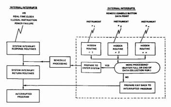
Figure 4. Diagram of software interrupt processing
