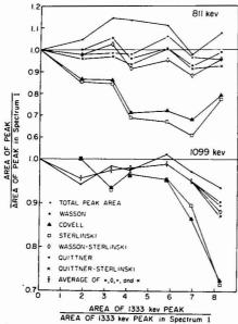
Figure 4. Variation in measured photopeak intensity for the 811-KeV and 1099-KeV photopeaks, for the seven methods studied, with increasing ©Co activity
