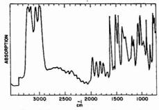
Figure 4. Spectrum of polystyrene (20-sec scan)
