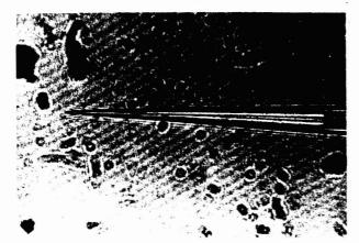
Figure 2. Photograph of a potassium liquid ion exchanger microelectrode with 125 microns of ion exchanger inside the tip. Magnification, 400×
