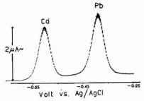
Figure 1a. Ac polarogram of  $8 \times 10^{-5}M$  Cd(II) and  $8 \times 10^{-6}M$  Pb(II) in 1M NaCl
