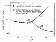
Figure 5. Ammonium ion suppression by addition of disopropylamine
