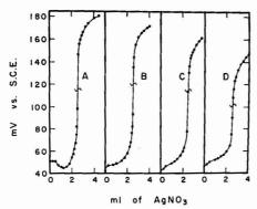
Figure 11. Titrations of 25 ml of 0.01 M KCl with AgNO<sub>2</sub> in the presence of varying concentrations of KNO<sub>2</sub>
