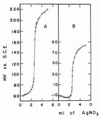
Figure 16. Titration of 25 ml of 0.01M KCl vs. AgNO<sub>3</sub> with different membranes
