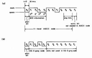
Figure 3. Current wave form for decimal three
