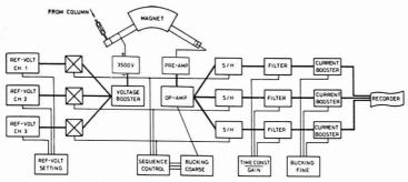
Figure 1A. Schematic diagram of the new multiple ion detector (MID)
