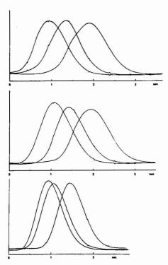
Figure 4. Recordings of single sweep cycles. The three peaks represent different molecular ions. The small spikes on two of the peaks are for channel identification. The y-axes represent ion intensities
