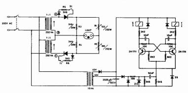
the vapor discharge lamp, this would mean that they could be driven correctly for instance, by inserting a rectifier in the circuit to suppress one half-period of the mains voltage, see Figure 2. The light output from this arrangement is shown in Figure 1, a, c. In all such arrangements the actual period of light emission is slightly shorter than the intervals of darkness. This usually does not impair the performance of a lock-in amplifier.
