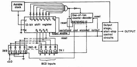
Figure 2. Functional diagram of P-S converter
