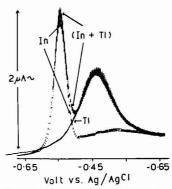
Figure 4. Diagram to show that observed ac wave in Figure 3b is the addition of the two ac waves in Figure 3a
