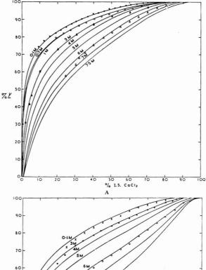
Figure 2. Selectivity isotherms for the Orion calcium activity electrode at constant ionic strength at 25 °C and pH  $\sim$ 7.5. Symbols represent experimental points
