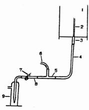
Figure 1. Connection to sample point of high temperature SO<sub>2</sub> reduction reactor
