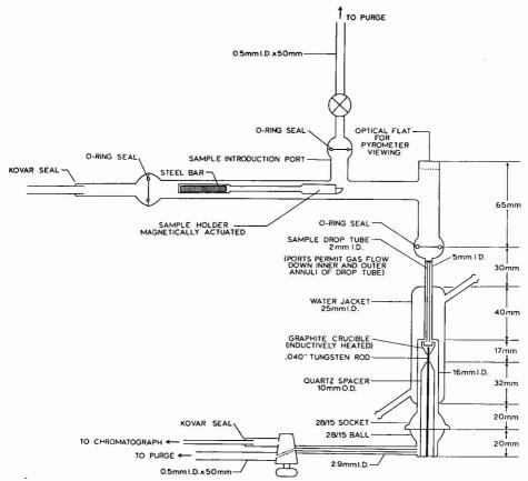
Figure 2. Fusion furnace detail
