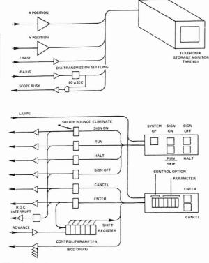
Figure 2. Simplified schematic of the interface to a remote operator's console On the top, the storage display scope and below, the console buttons and thumbwheel digits
