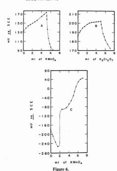
Titration of 50 ml of 0.01M FeSO<sub>4</sub> (NH<sub>4</sub>)<sub>2</sub>SO<sub>4</sub> vs. KMnO<sub>4</sub>
