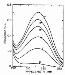
Figure 1. Absorption spectra showing formation of  $\alpha$ -benzamidobenzyl-penicillenic acid after addition of excess benzoyl chloride and acid treatment
