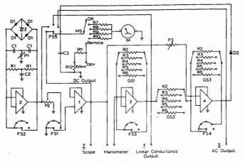
Figure 3. Circuit diagram of pressure transducer system
