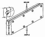
Figure 3. IR-GC spectrometer gas cell
