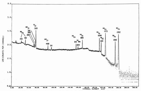
Figure 2. Gamma-ray spectrum of the Allende chondrite, two weeks following irradiation
