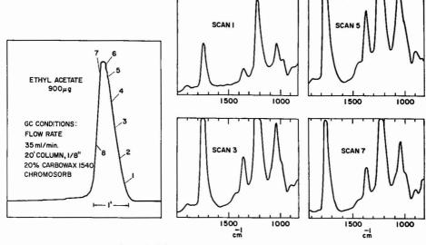
Figure 10. Infrared spectra of ethyl acetate as GC fraction
