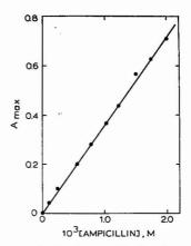
Figure 4. Absorbance as a function of ampicillin concentration, assayed under optimum conditions
