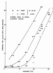
Figure 3. Plot of phase-insensitive corrosion maxima in 30% NaOH solution vs. manganese content for a number of alloys Corresponding aluminum content for each specimen is recorded and the 5, 10, and 15% aluminum contours roughly drawn in
