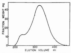
Figure 1. Weight distribution of fractions separated from the asphalt by GPC
