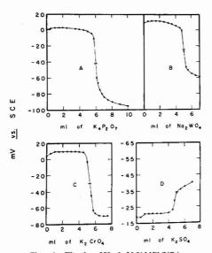
Figure 1. Titration of 50 ml of 0.01 M Pb(NO2)2
