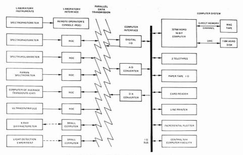
Figure 1. Diagram of the laboratory-based computer system
