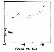
Figure 3. Derivative pulse polarogram of  $4 \times 10^{-8}M$  Cd<sup>2+</sup>,  $5 \times 10^{-4}M$  KNO<sub>3</sub>
