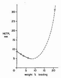
Figure 2. Variation of plate height (HETP) with weight percentage loading of DNP on Teflon for ethanol solute at 86 °C
