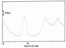
Figure 7. Derivative pulse polarogram of  $4 \times 10^{-6} M \text{ Cd}^{2+}$ ,  $0.05 M \text{ KNO}_3$
