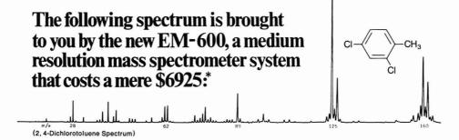
Before leaving, we might mention that the 60° sector, magnetically scanned EM-600 is a complete, easy-to-use system which also features a heated inlet for volatile organic compounds up to mass 330 or higher and linear mass readout.
