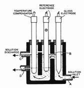
Figure 6. Cell arrangement
