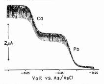
Figure 1b. Dc polarogram of same solution as in 1a
