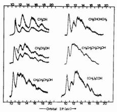
Figure 1. Photoelectron spectra of some aliphatic alcohols, excited by irradiation with 584-Å photons
