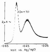
Figure 3b. Ac polarogram of  $8\times 10^{-6}M$  Tl(I) and  $4\times 10^{-6}$  In(III) when both are present in the one solution
