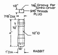
Figure 4. Schematic of polyethylene-boron rabbit
