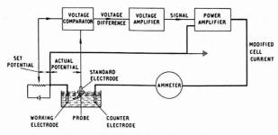
Figure 1. Working principle of the potentiostat
