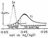
Figure 3a. Ac polarograms of  $8 \times 10^{-6}M$  Tl(1) and  $4 \times 10^{-6}M$  In(III)
