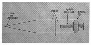
Figure 1. Schematic diagram of an ion specific liquid ion exchanger microelectrode
