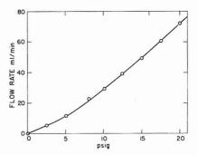
Figure 2. Typical calibration curve for ceramic gas dilution device
