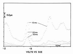
Figure 6. Derivative pulse polarogram of 4  $\times$  10<sup>-6</sup>M Cd<sup>2+</sup> 0.05M KNO<sub>3</sub>
