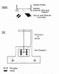
Figure 2. Schematic of external wire. (a) Location; (b) wire holder
