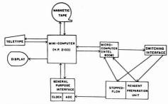
Figure 1. Block diagram of computer controlled stopped-flow system
