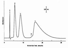
Figure 1. Chromatogram of tetracycline hydrochloride containing 0.6% (4*R*)-anhydrotetracycline and ∼0.75% (4*S*)-anhydrotetracycline, detection at 429 nm
