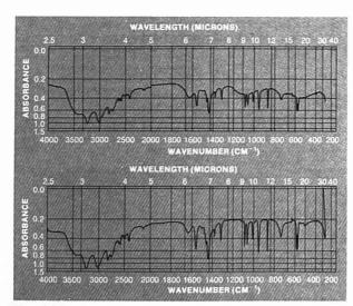
Figure 3. Infrared spectra of: upper: solids from naphtha reboiler furnace tubes; lower: tars formed on heating HCl salts of corrosion inhibitor
