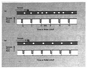
Figure 5. Sample proportioning as function of air bubble injection (a) Air segmentation with no air-bar (b) Air segmentation with air-bar timed at roller liftoff
