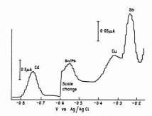
Figure 5. DPASV curves for Cd, Cu, and Sb in plant zinc sulfate solution diluted 1:1 with concentrated HCl
