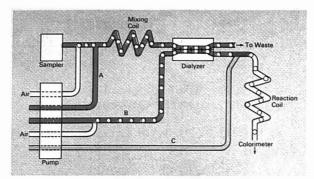
Figure 1. Example of continuous-flow analysis scheme A, B: diluents; C: reagent stream
