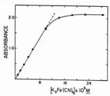
Figure 7. Absorbance vs. concentration for potassium ferricyanide solutions and measured by the automated stopped-flow system
