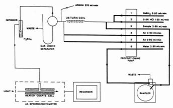
Figure 1. AutoAnalyzer-AAS system for tin
