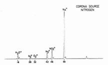
Figure 2. Mass spectrum of nitrogen obtained with the corona discharge point located at a distance of 0.5 mm from the sampling aperture. Source temperature, 200 °C
