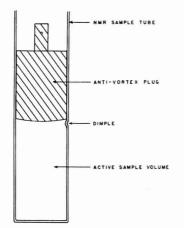
Figure 1. Diagram of anti-vortex plug in an NMR sample tube
