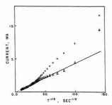
Figure 1. Current-time curve for potentiostatic reduction of methyl viologen
