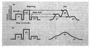
Figure 2. Effect of dispersion during continuous-flow analysis on sample concentration curve shape
