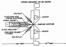
Figure 1. Schematic diagram of a corona discharge source with an adjustable distance between point and sampling aperture
