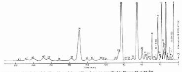
Figure 11. Chromatogram of the industrial still residue mixture with column as specified in Figure 10 at 75 °C
