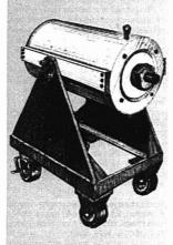
For subjecting samples to pure hydrostatic pressures up to 10 kilobars and temperatures up to 1400°C simultaneously. Tem-Pres offers a variety of pressure vessels with a furnace located inside the vessel housing. Easily replaceable, cartridge-type furnaces, with dual control zones, allow complete control of hot-zone location.
