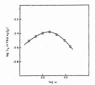
Figure 4. Effect of  $\omega$  on simulated current. Parameters used:  $k_3C_{\rm E}/K_{\rm m}$  = 1.  $C/K_{\rm m}$  = 0.01
