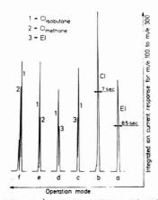
Figure 3. Chromatograms of the integrated ion current of pentobarbitone at different modes of operation
