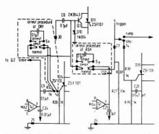
Figure 1. Circuit modifications which permit interruption of the analytical cycle are enclosed within dotted lines
