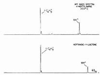
Figure 6. API mass spectra of reaction products for n-heptylamine and heptanoic-γ-lactone in the presence of t-C<sub>4</sub>H<sub>9</sub>+ at 200 °C (<sup>63</sup>Ni source)
