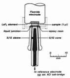
Figure 5. Detail of the fluoride electrode and sleeve-junction in use
