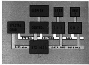
Figure 1. Multichannel asynchronous serial transmitter Block diagram shows two instruments connected to two active channels
