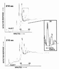
Figure 6. Replicate chromatograms of a No. 2 fuel oil
