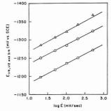
**Figure 4.** Dependence of the characteristic potentials ( $\square$   $E_{1/4}$ , O  $E_{1/2}$ , and  $\triangle$   $E_{3/4}$ ) on the logarithm of the ramp-rate. Conditions as in Figure 3
