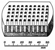
Figure 1. Polypropylene block used to prepare test solutions from samples soluble in 1 M perchloric acid. The curved ends of the block enable it to be centrifuged within the 250-ml bucket of a preparative centrifuge
