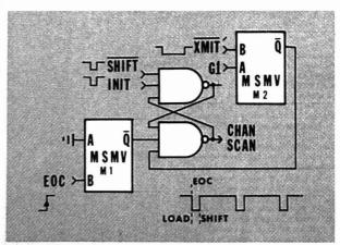
Figure 5. Channel scanner
