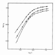
Figure 1. Experimental steady-state disk current ( $I_D(\mu A)$ ) as a function of glucose concentration (M) at various electrode rotation speeds: 400 rpm ( $\Delta$ ), 900 rpm ( $\Box$ ), and 1600 rpm (+)
