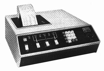
relative response factor, area % and normalized area %. Through powerful file linking, any combination of these methods can be automatically applied to the data from a single injection and the results automatically reported in more than one form, e.g., weight %, mole % and volume %.
