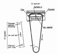
Figure 1. Schematic drawing of the combined EI/CI ion source
