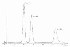
Figure 2. Separation of Cu(en)AA, Cu(tm)AA, and Cu(en)BA. Column: MicroPak CH; mobile phase: methanol/phosphate buffer pH 7.8, 50/50 (v/v). Flow rate: 1 cm<sup>3</sup> min<sup>-1</sup>. Theoretical plate number for Cu(en)BA: 940
