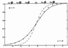
Figure 1. Comparison of the shape of an irreversible neopolarogram (full line) with a reversible (neo)polarogram (dashed line) and an irreversible polarogram (unconnected points)
