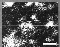
Auger Image showing distribution of nickel on surface of methanation catalyst.
