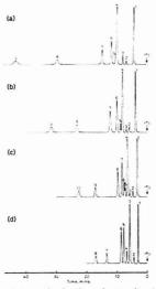
Figure 5. Chromatograms showing the major constituents of an industrial still residue mixture at 100 °C with columns of: (a) di-n-nonyl phthalate (DNNP); (b) squalane and DNNP ( $\phi=0.6276$ ); (c) squalane and DNNP ( $\phi=0.3315$ ); (d) squalane
