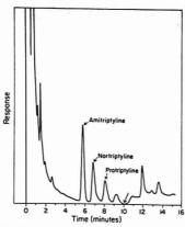
Figure 1. Gas-liquid chromatogram of blank serum with (20 ng/ml) of amitriptyline, nortriptyline, and protriptyline added after the serum was carried through the extraction
