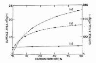
Figure 4. BET surface area (N<sub>2</sub>, 77 K) vs. burn-off (a) Coke. (b) Electrode graphite. (c) Nuclear graphite
