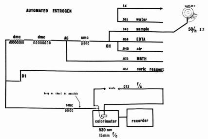
Figure 1. Manifold diagram for automated color development
