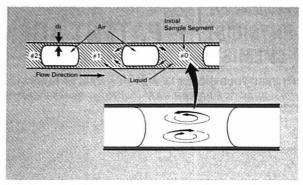
Figure 3. (a) Sample dispersion during segmented flow through open tube with marker-dye sample injected into segment #0. Film of liquid phase ( $d_r$  = film thickness) from segment #0 will be overtaken and mixed into segment #1, allowing dye to move from #0 to #1; dye built up within segment #1 can also be transferred to #2. Dye will become dispersed over many following segments. (b) Bolus circulation within moving liquid segment occurs naturally in any segmented-flow system
