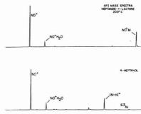
Figure 8. API mass spectra of reaction products for a secondary alcohol and for a lactone in the presence of NO<sup>+</sup> at 200 °C (<sup>63</sup>Ni source)
