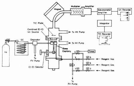
Figure 2. Schematic diagram of the combined gas chromatograph-mass spectrometer and reagent gas inlet system for EI/CI operation
