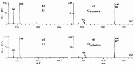
Figure 4. Mass spectra of pentobarbitone obtained from GC peaks c and d (Figure 3)
