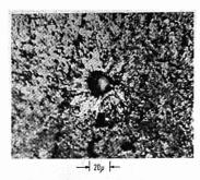
Figure 3. Single shot ruby laser crater in steel
