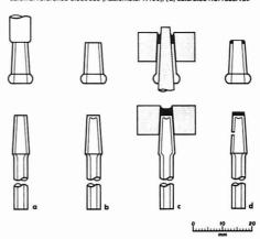
Figure 4. Stages in the construction of the ground-sleeve junction
