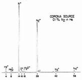
Figure 3. Mass spectrum of 0.1% nitrogen in hellum, obtained with the corona discharge point located at a distance of 0.5 mm from the sampling aperture. Source temperature, 200 °C
