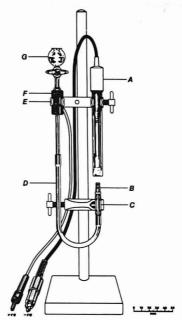
Figure 3. Fluoride electrode assembly
