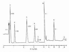
Figure 2. Typical chromatogram of pyrolysis gas
