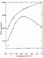
Figure 2. Dependence of oxidation rate of carbon on percentage
