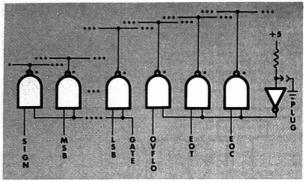
Figure 3. Data bus routes input data into STX 1003 parallel inputs and control indicators into appropriate control logic
