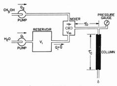
Figure 1. Model LC oscillator with single reservoir
