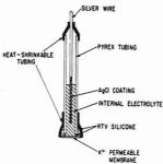
Figure 1. Construction of the electrodes
