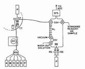
Figure 2. Schematic representation of automated stopped-flow system
