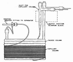
Figure 1. Dual column arrangement
