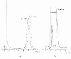
Figure 3. (a) Superimposed chromatograms of Cu(en)BA and Ni(en)BA. Column: MicroPak CH; mobile phase: methanol/phosphate buffer pH 7.0, 70/30 (v/v). Flow rate: 1.5 cm³ min⁻¹. (b) Separation of Cu(en)BA and Ni(en)BA. Column: –NH<sub>2</sub> 50 cm × 0.2 cm; mobile phase: methanol/phosphate buffer pH 7.8, 40/60 (v/v). Flow rate: 1 cm³ min⁻¹. Theoretical plate number for Ni(en)BA: 346
