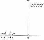
Figure 4. Mass spectrum of 0.1% argon in helium obtained with the corona discharge point located at a distance of 0.5 mm from the sampling aperture. Source temperature, 200 °C
