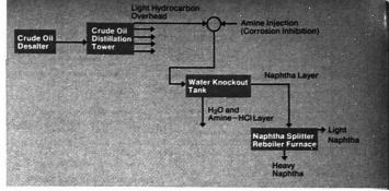
Figure 1. Block diagram of portion of refinery involved in crisis
