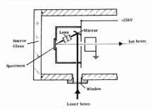
Figure 1. Mass spectrometer source arrangement
