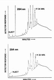
Figure 3. Chromatograms of two No. 6 fuel oils refined from the same feedstock
