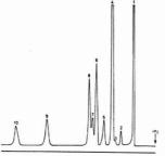
Figure 7. Chromatogram of the industrial still residue with a column of  $\phi_{\text{DNNP}}=0.0749$ ; other conditions as specified in Figure 5
