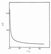
Figure 2. Simulated current transient at rotating disk electrode time (s) after application of potential, t. Steady-state current,  $I_{\rm e}$ . Other parameters LT=300, DM=0.45,  $\omega=400$  rpm, V=0.2266, and  $C/K_{\rm m}=1$  are defined in text
