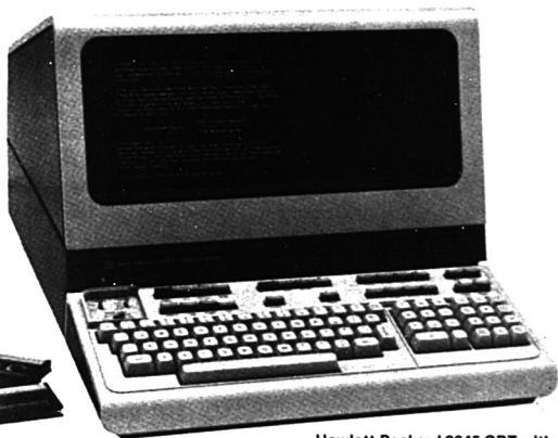
Hewlett-Packard 2645 CRT with dual cartridges to optimize software flexibility.
