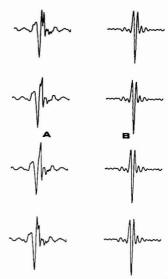
Figure 6. Four successive single-scan interferograms in the region of zero retardation, (A) measured dual-beam and (B) measured single-beam; both sets of data were measured using a TGS detector
