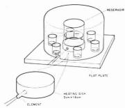
Figure 1. Reagent chamber transfer apparatus
