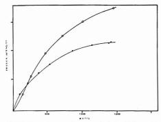
Figure 3. Comparison of radiant output of pulsed and CW operated Ar EDLs as a function of incident rf power; no high intensity mode occurring. (O) pulsed operation, (▲) CW operation. In the pulsed mode, the signals recorded are peak values
