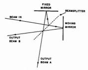
Figure 1. The two output beams (A and B) from a Michelson interferometer when the input beam is slightly skewed
