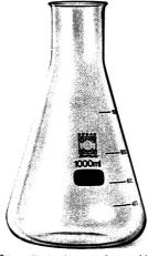
DURAN® borosilicate glassware is superbly finished, has uniform wall thicknesses and doesn't lose its cool when the thermometer climbs to 500 °C. It conforms with the international standard ISO 3585.
