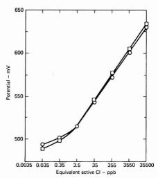
**Figure 7.** Simultaneous computer-based calibration of two Orion 97-70 residual-chlorine electrodes with chloramine-T in pH 4 buffer. Slopes are 30.0 and 29.55 mV per decade of concentration
