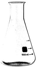
Brand X borosilicate glassware is superbly finished, has uniform wall thicknesses and doesn't lose its cool when the thermometer climbs to 500 °C. It conforms with the international standard ISO 3585.
