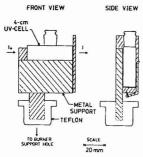
Figure 1. Cell holder attachment for stationary cold-vapor atomic absorption measurements
