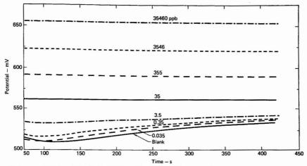
Figure 3. Response of the Orion 97-70 chloride electrode to chloramine-T in pH 4 acetate buffer
