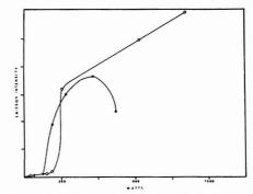
Figure 4. Comparison of radiant output of pulsed and CW operated Hg EDLs as a function of incident rf power. (O) pulsed operation, (O) CW operation. In the pulsed mode, signals recorded are peak values
