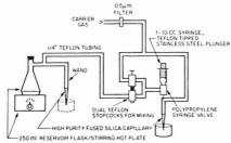
Figure 2. Gas stream transfer apparatus
