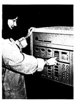
Model 150C liquid chromatograph/gel permeation chromatograph is a high-speed, controlled-temperature instrument. Known as "The Hot One", the instrument provides rapid results, with separations in 7-15 min. Operation is microprocessor controlled. The Model 150C will analyze materials that dissolve only at elevated temperatures or require high temperatures to reduce viscosity. Waters Associates, Inc. 402
