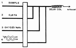
Figure 1. Flow system design
