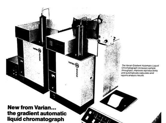
Now, the high performance Varian 8500 series offers both an Isocratic and a Gradient Automatic Liquid Chromatograph. The new Automatic Gradient Liquid Chromatograph will run up to 60 gradient analyses unattended for 16 or more hours and it will run isocratic analyses for an even longer period. Everything is automatic: injection, separation, calculations and final report.
