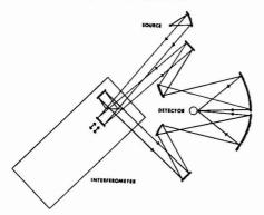
Figure 2. Optical diagram of the dual-beam Fourier transform spectrometer used in this work
