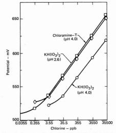
Figure 2. Computer calibration of an Orion 97-70 residual-chlorine electrode under three different conditions
