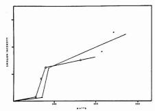
Figure 6. Comparison of radiant output of pulsed and CW operated Zn EDLs as a function of incident rf power. (X) pulsed operation. (O) CW operation. In the pulsed mode signals recorded are peak values
