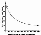
Figure 8. The relative S/N for the 2875 cm-1 polyethylene band measured with the dual-beam optics using the MCT and TGS detectors, as a function of the percentage of the source radiation entering the interferometer
