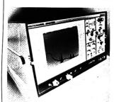
Series 30 multichannel pulse height analyzer features a 9-in. diagonal CRT, 1024 channel memory, and both PHA and MCS data acquisition modes. Digital integration, spectrum compare, and I/O interfacing for TTY, EIA devices and digital cassette are included in the basic unit. Plug-in options are available for a detector bias supply, high-resolution amplifier, and various additional I/O interfaces. Canberra Industries, Inc. 404
