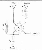
Figure 1. Diagram of the liquid chromatograph (description in text)
