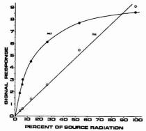
Figure 7. Maximum intensity of the 2875 cm<sup>-1</sup> polyethylene band measured using the dual-beam optics as a function of the percentage of the radiation from a modified Nernst glower source using the MCT detector ( ) and TGS detector (O). The nonlinearity of the response of the MCT detector is evident. (The ordinate scale for the MCT detector is ten times larger than that for the TGS detector)
