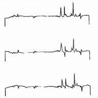
Figure 5. Three successive single-scan spectra from 3200-800 cm<sup>-1</sup> of a 0.1% solution of anisole in CCl<sub>4</sub> (90-µm pathlength) with a cell of equal thickness filled with pure CCl<sub>4</sub> in the reference beam, showing the difficulty in phase correction
