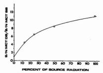
Figure 9. Calculated ratio of the relative S/N of the 2875-cm-1 polyethylene band measured using an MCT detector in the dual-beam and single-beam configurations, as a function of the source radiation entering the interferometer
