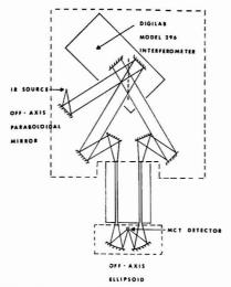
Figure 1. Optical layout of the dual-beam system for the on-line measurement of GC peaks
