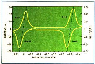
Figure 2. —, left axis. Cyclic voltammogram of 1.3 mM Co<sup>n</sup>(sal<sub>2</sub>en) in 0.5 M tetraethylammonium perchlorate-dimethylformamide. Optically transparent thin-layer electrode with gold minigrid. Scan rate 2 mV s<sup>-1</sup>. —, right axis. Nernstian plots of log ([red]/[ox]) vs. E<sub>applied</sub> for Co<sup>m</sup>, Co<sup>m</sup> and Co<sup>m</sup>, Co<sup>m</sup> couples
