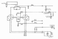
Figure 1. Circuit diagram of rf generator
