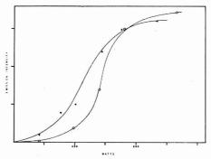
Figure 2. Comparison of radiant output of pulsed and CW operated Ar EDLs as a function of incident rf power. (O) pulsed operation, ( $\Delta$ ) CW operation. In the pulsed mode, the signals recorded are peak values
