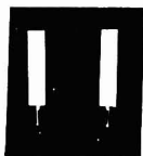
Figure 2. X-ray of two capillaries filled with mercury
