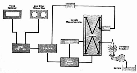
Figure 7. Schematic diagram of a programmable ICP scanning spectrometer
