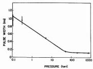
Figure 6. Absorption pulse width (ms) measured at 10% of maximum absorption vs. pressure for Mn atomic absorption in a NBS 461 steel sample
