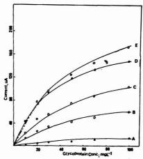
Figure 5. Glycoprotein calibrations at pH 1.67 in the DPP mode at 60  $S\,h^{-1}$  with varying TiO<sup>2+</sup> reagent concentrations: (A) 2.0  $\times$  10<sup>-2</sup>, (B) 3.0  $\times$  10<sup>-2</sup>, (C) 4.0  $\times$  10<sup>-2</sup>, (D) 5.0  $\times$  10<sup>-2</sup>, (E) 6.0  $\times$  10<sup>-2</sup> M
