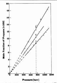
Figure 1. Partition isotherms for propane in *n*-hexadecane at 25, 35, and 45 °C. Literature data at 760 Torr. (\*) Hayduk et al. (28, 31). (Δ) King and Al-Najjar (30). (□) Chappelow and Prausnitz (29)
