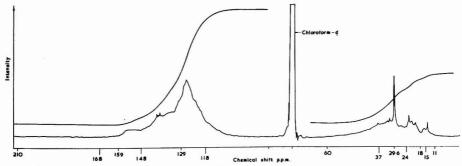
Figure 1. 13C spectrum of asphaltenes from a hydrogen donor solvent extract (extract a)
