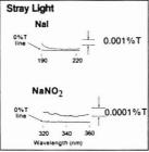
Measured stray light on a typical High Performance 559 (shown above) is well within the specification of 0.002%T at 220 nm and 0.001%T at 340 nm.
