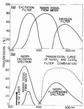
Figure 3. Transmission curves: (a) for a conventional fluorimeter; and (b) for the laser fluorimeter. The excitation and fluorescence spectra of NADPH are shown in (b). The Raman signal for each setup is also presented
