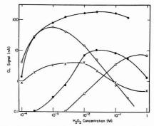
Figure 2. Variation of CL signal with  $H_2O_2$  concentration. Lophine =  $3.25 \times 10^{-4}$  M; KOH = 0.20 M. OCl<sup>-</sup> ( $\blacksquare$ ), Cu(II) (O), Cr(III) ( $\blacksquare$ ), Co(II) ( $\square$ ), VO<sup>2+</sup> ( $\times$ )
