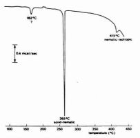
Figure 1. DSC scan of BPhBT, scan rate 10 °C/min, helium flow rate 50 mL/min
