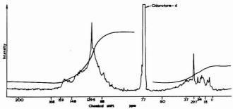
Figure 2. <sup>13</sup>C spectrum of asphaltenes from a supercritical gas extract (extract b)
