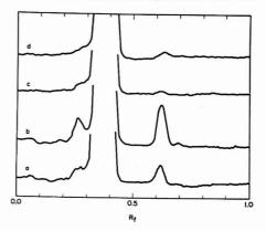
Figure 2. Swishing monitored by TLC: (a) original sample, (b) swish solution residue, (c) purified solid from 1-g swish, (d) purified solid from 100-g swish
