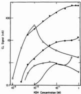
Figure 4. Variation of CL signal with KOH concentration. Lophine =  $3.25 \times 10^{-4}$  M;  $H_2O_2 = 1.0 \times 10^{-1}$  M. OCt ( $\blacksquare$ ), Cu(II) ( $\square$ ), Vo<sup>2+</sup> ( $\times$ )
