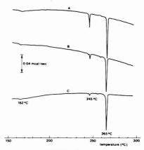
Figure 2. DSC scans of BPhBT on Chromosorb WHP of one sample
