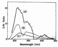
Figure 3. S/N ratio of fluorescein (pH 13,  $5 \times 10^{-11}$  M). Excitation source: (A) esculin dye laser (480 nm), (B) 4-MU dye laser (450 nm), (C) Al-Calcein Blue chelate laser (420 nm)
