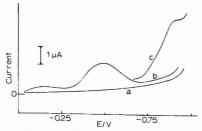
Figure 1. Linear potential scan voltammetry of nitrite at Hg in the catalytic medium. (a) 0.1 M KCl; pH 2.1 (presence or absence of nitrite). (b) 0.1 mM MoO<sub>4</sub><sup>2-1</sup>; 0.1 M KCl; pH 2.1. (c) 0.3 mM NO<sub>2</sub><sup>-1</sup> in b. (Curves b and c superimpose in region not shown. Scan rate, 70 mV·s<sup>-1</sup>. The pH was adjusted with dilute HCl
