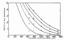
Figure 6. Concentration vs. distance for five times during forward step of double-potential step experiment. Theoretical curves from the top: 5, 4, 3, 2, 1s. Experimental points:  $(\Delta)$  5 s, (0) 4 s,  $(\square)$  3 s,  $(\Delta)$  2 s,  $(\Phi)$  1 s
