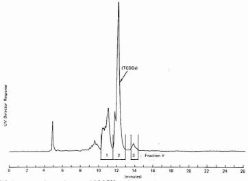
Figure 6. RP-HPLC chromatogram for caustic extracted 2,3,6-TCP pyrolyzate, conditions in text
