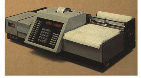
tant application, a sample of grain, such as wheat, corn, or soybeans, is ground to a powder and packed into a cup. The sample cup is placed in a filter reflectance spectrophotometer, and the instrument measures reflectance at six wavelengths in the near infrared. The instrument then solves three simultaneous equations to compute percentages of protein, oil, and moisture in the grain. The whole procedure takes about one minute.
