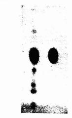
Figure 3. Enrichment of TLC impurities: left, original sample; right, swish solution residue
