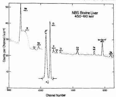
Figure 5. Prompt γ-ray spectrum of NBS Bovine Liver (SRM 1577) in the region of 450 to 610 keV observed by irradiating a 1.3-g sample for 24 h in the external thermal-neutron beam of the NBS reactor. Peaks are labeled by energies in keV and the element of origin
