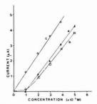
Figure 5. Cathodic stripping of compound I with electrolyte (0.05 M KNO<sub>2</sub>/HNO<sub>2</sub>) presaturated with mercurous chloride. Electrolyte (a) with no mercurous chloride; (b) presaturated cold with mercurous chloride; (c) presaturated at 70 °C with mercurous chloride
