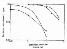
Figure 7. Suppression of the analytical CL signal as a function of the ratio of the concentrations of the interfering species and the analyte. All analytes are at 10-4 M. The reagent concentrations are chosen from Table IV for the analyte. Cu(II) analyte, Cr(III) interference (O); Cr(III) analyte, Cu(II) interference (●); Cu(II) analyte, Co(II) interference (□); Co(II) analyte, Cu(II) interference (■)
