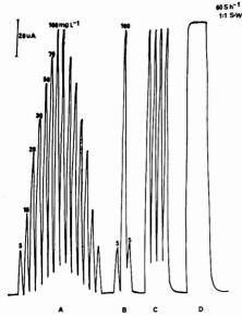
Figure 7. Continuous recording of glycoprotein sample peaks at a fixed potential of ~0.55 V. (A) Calibration for the concentration range 5–100 mg L<sup>-1</sup>. (B) Carryover between sequential samples of 5, 100, and 5 mg L<sup>-1</sup> glycoprotein. (C) Replicates for 100 mg L<sup>-1</sup> glycoprotein; (D) steady-state reading at 100 mg L<sup>-1</sup>
