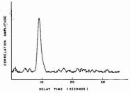
Figure 7. Same correlation chromatogram as in Figure 6, except that carrier frequency was reduced to 0.303 Hz. Correlation noise is greatly reduced because one complete PRBS code is used
