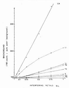
Figure 1. Action of different metals on the background measured at the peak base of aluminum line: 396.09 nm
