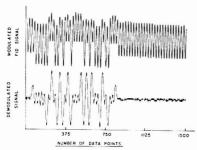
Figure 2. Detector output and demodulated signal of hexane on Durapak-N-octane at 60 °C. PRBS code length = 31. Data acquisition rate = 10 Hz. Carrier frequency = 0.400 Hz. Flow rate = 40 cm³/min. Column head pressure 18 psi. Modulation bandwidth = 0.416-0.384 Hz. or ±4.0 %
