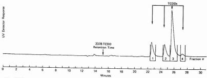
Figure 8. Silica-HPLC chromatogram for RP-HPLC TCDDs fraction #2, conditions in text
