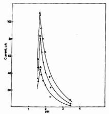
Figure 4. Effect of pH on the continuous-flow peak heights for gly-coprotein at fixed TiO $^2$ \* and oxalic acid concentrations. TiO $^2$  (5.0  $\times$  10 $^2$  M), oxalic acid (4.0  $\times$  10 $^2$  M) with glycoprotein concentrations of: (A) 10, (B) 20, and (C) 70 mg L $^{-1}$
