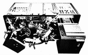
The 70-70H high resolution mass spectrometer has a resolution of 25 000 and a mass range of 2 to 700 at 4kV. The 70-70H is capable of scan rates of up to 0.3 sec./decade. The scan cycle time over the mass range 500 to 25 is 0.8 sec., so the 70-70H is suitable for high resolution capillary GC/MS. A data system which includes extensive control facilities can be supplied. VG-Micromass
