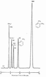
Figure 2. Chromatogram of alkyliodides. Column 10-ft UC W98 methyl silicone; helium 20 mL/min. Temperature 100 °C: 170 mA grammed to report weight percent alkoxyl by entering the internal standard and sample weights.
