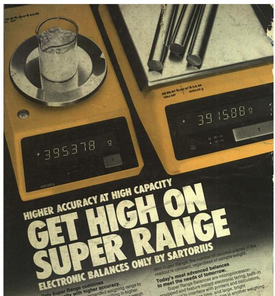
Only Super Range combines high capacity with higher accuracy. Super Range is an expanded weighing range to the full capacity of the balance, resulting in higher readout accuracy. With Super Range, you can weigh 400 grams to 0.001g (Model 1265MP, above left), or 4,000 grams to 0.01g (Model 1260Mr. apove 19th).
