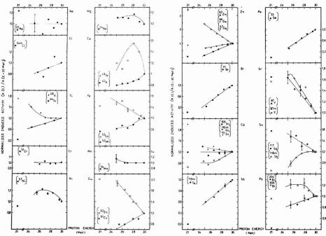
Figure 1. Relative excitation functions for the production of radionuclides from irradiation of natural elements with 21 to 30 MeV protons
