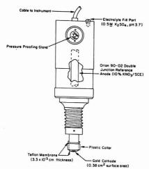
Figure 1. Schematic view of the membrane electrode system
