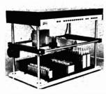
MultiRac is a microprocessor-controlled fraction collector suitable for use even with organic solvents and radioactive liquids. Collection can be made according to time, drop, or precise volume. Volume size can be varied from 10 µL to 3500 mL. Trays accept both funnels and spring-loaded racks which accommodate a variety of vessels from 12 mm diameter test tubes to 28 mm diameter scintillation vials. Data show on a red LED display. \$2995. LKB Instruments, Inc. 404
