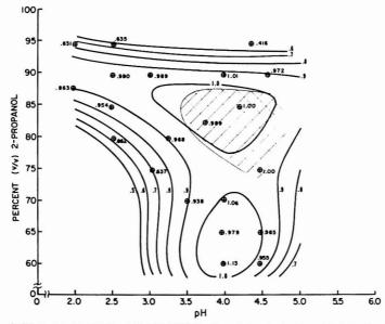
Figure 3. Fraction of sulfate recovered as a function of pH and % PrOH. Experimentally determined points are indicated by  $\oplus$ , with the corresponding fractional recovery. Cross-hatching indicates region of sharpest end points.
