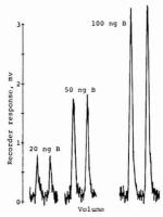
Figure 5. ICP detection of boron peaks at three different concentrations (two peaks for each concentration) enabled calculation of the detection limit, denoted as minimum detectable concentration (MDC), given in Table IV.
