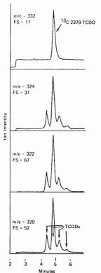
Figure 7. Packed column GC-LRMS mass chromatograms for RP-HPLC TCDDs fraction #2, conditions in text. FS is full scale factor applied to each ion
