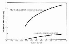
Figure 6. Plate height vs. velocity for poly(N,N-diallyldimethylammonium chloride) and N,N-dimethylpiperidinium chloride in 0.1 N HNO<sub>3</sub> + 0.1 N NaNO<sub>3</sub> on a 10-column set of quaternized supports varying in porosity from 40 to 25 000 Å
