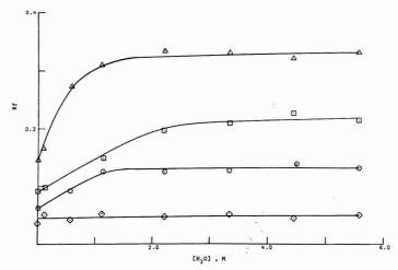
Figure 3. A plot of *R*<sub>1</sub> value vs. concentration of water (in the sodium dioctylsulfosuccinate reversed micelle) for uridine (Δ), cytidine (□), guanosine (Θ), and adenosine (♦)
