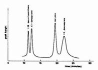
Figure 5. Resolution of PAH on a packed column. Column conditions: 8 ft, 1.8-mm i.d., helium flow 20 mL/min
