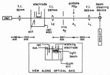
Figure 1. Schematic of experimental apparatus. Laser is a 0.5-mW He-Ne (Spectra Physics, Mountain View, Calif.), PMT is a 1P28. Beam was directed into L, by a beam steering device (Newport Research, Fountain Valley, Calif.). The long axis of the slit was oriented perpendicular to the plane of the figure, immediately to the left of the electrode. Insert shows details of cell, viewed along the optical axis, in the direction of light propagation
