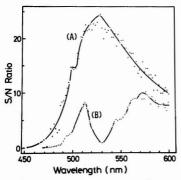
Figure 5. S/N ratio of riboflavin (pH 6-7, 1 imes 10<sup>-9</sup> M). Excitation source: (A) PBD dye laser (377 nm), (B) 4-MU dye laser (450 nm)
