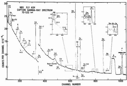
Figure 1. Prompt γ-ray spectrum of NBS Fly Ash (SRM 1633a) in the region of 70 to 520 keV observed by irradiating an 0.82-g sample for 20 h in the external thermal-neutron beam from the NBS reactor. Peaks are labeled by energies in keV and the element of origin
