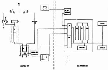
Figure 1. Schematic of coupling elemental analyzer-data processing unit. (1) Flow controller, (2) oxygen injection valve, (3) sample holder, (4) reactor, (5) furnace, (6) GC column, (7) thermostatic oven, and (8) recorder
