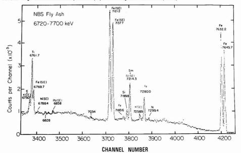
Figure 4. Prompt γ-ray spectrum of NBS Fly Ash (SRM 1633a) in the region of 6720 to 7700 keV. See caption of Figure 3
