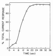
Figure 6. Response time to step change from 0 to 1 mg/L ozone at stirring rate of 1000 rpm
