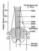
Figure 5. Schematic representation of a typical ICP used in analytical spectroscopy
