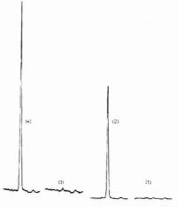
Figure 2. Spectra obtained for wavelength sweeps from 395.90 to 396.35 nm with pure water (1), pure water containing 250  $\mu$ g/L AI (2), 250 mg/L Ca (3), 250  $\mu$ g/L AI + 250 mg/L Ca (4)
