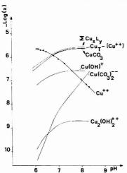
Figure 7. Copper carbonate and hydroxo complex distribution as a pH function.  $Cu_T = 2.62 \cdot 10^{-6} \text{ M}; C_T = 2.47 \times 10^{-3} \text{ M} [Ca(HCO_3)_2];$   $L = OH^- \text{ or } CO_3^{2-}; x = 1 \text{ or } 2; y = 1 \text{ or } 2$
