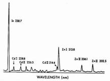
Figure 4. Spectrum of 0.0001% G-7 Spex Industries graphite matrix powder standard
