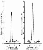
Figure 2. AAS and ICP detector response to 100 ng Cu chelated to NTA in a 10- $\mu$ L sample run through the dummy HPLC column. For AAS, peak height/noise, 26.6; fwhrm. 0.40 cm; peak area, 5.3 cm²; noise, 0.50 cm. For ICP, peak height/noise, 23.1; fwhm 0.55 cm; peak area, 10.6 cm²; noise, 0.85 cm
