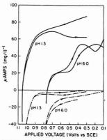
Figure 2. Current-voltage relationship at the rotating gold electrode in 0.05 M H<sub>2</sub>SO<sub>4</sub> (pH 1.3) and 1.6 M KCl (pH 6.0). Solid lines are for ozone reduction current and dashed lines are residual current
