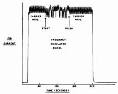
Figure 5. Entire detector output for an FM experiment (carrier > FM > carrier). Same conditions as Figure 2
