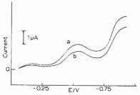
Figure 2. Effect of electrode-solution contact time on the generation of the catalyst. (a) 0.5 min of Hg-solution contact at 0.0 V prior to LSV. (b) LSV scan initiated immediately after contact of the Hg electrode to the solution. All other conditions the same as in Figure 1c
