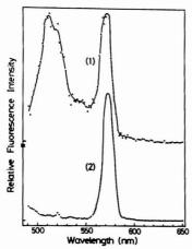
Figure 1. Fluorescence spectrum of fluorescein (pH 13,  $5 \times 10^{-11}$  M) (1) and background spectrum of solvent water (2). Excitation source: esculin dye laser ( $\lambda_{\rm ex} = 480$  nm,  $\Delta\lambda_{\rm ex} = 0.3$  nm)
