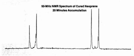
\*\*C spectrum of cured neograms with carbon black\* in a Kel F rotor using high power gated decoupling (400 transients at 3 second intervals). The resolution has been enhanced by a Lorentzian to Gaussian transformation to bring out the fine structure. The width of the plot is 10 kHz. \*\* Sample courtesy of E + Du Port de Nemours and Company.
