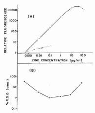
Figure 3. ICAP-excited AFS analytical growth curve (A) and precision curve (B) for zinc in a nitrogen-separated air/acetylene flame at 213.9 nm
