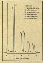
Separation of a mixture of free steroids on a 3 ft.OV-17 SERIES 3000-3 HI-EFF column.
