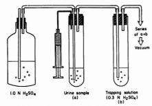
Figure 1. Schematic diagram of the aeration train. The syringe attached to the sample tube contains saturated K2CO3, which is to be injected into the sample
