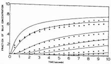
Figure 3. Fraction of bulk concentration vs. time at various distances from the electrode for a single-step experiment. Solid lines are theoretical curves (listed from top) at 25, 38, 70, 102, 133, 197, and 260 μm from the electrode. Points are experimental results: (●) 25 μm, (■) 38 μm, (▲) 70 μm, (◊) 102 μm, (Ο) 133 μm, (□) 197 μm, (Δ) 260 μm
