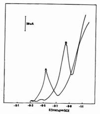
Figure 3. Effect of high glycoprotein concentration on the continuous-flow differential pulse scan of potassium titanium oxalate reagent solution. (A) Reagent alone  $(5.0 \times 10^{-2} \, \mathrm{M})$ : (B) reagent with added glycoprotein  $(1000 \, \mathrm{mg \, L^{-1}})$
