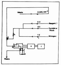
Figure 1. Schematic diagram of the polarographic flow system. (a) Flow-through cell; (b) Pt auxillary electrode; (c) SCE; (d) waste electrodyte solution; (e) PAR model 174; (f) recorder; (g) debubbler; (h) mixing coil; (i) proportioning pump; (j) potassium titanium oxalate reagent (5.0 × 10<sup>-2</sup> Mi) n 4.0 × 10<sup>-2</sup> M oxalic acid at ph 1.67
