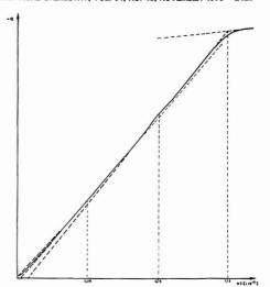
Figure 2. Typical thermogram obtained during neutralization of a citric acid solution ( $C_A = 7.20 \times 10^{-3} \text{ mol L}^{-1}$ ,  $V_0 = 10^{-1} \text{ L}$ ) by a sodium hydroxide solution ( $C_B = 1.91 \text{ mol L}^{-1}$ )
