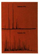
Figure 4. Coal Hydrogenation Product. In the analysis of very complex samples such as this coal hydrogenation product the 3700's capillary system gives high resolution of sample components. The capillary effluent splitter permits detection of the sulfur compounds with the FPD and the organics with FID.
