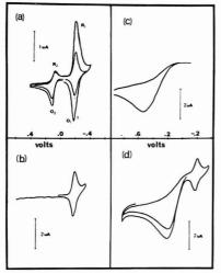
Figure 5. Oxo-apomorphine-modified carbon paste electrode. Buffer, pH 6.8 phosphate; scan rate, 3 V/min. (a) Fresh carbon paste electrode after 1st and 5th scans, immersed in 1 × 10-4 M apomorphine; (b) "chemically modified" electrode immersed in buffer only; (c) fresh carbon paste electrode immersed in 1 × 10<sup>-3</sup> M ascorbic acid; (d) "chemically modified" electrode, as in (b), immersed in 1 × 10-3 M ascorbic acid
