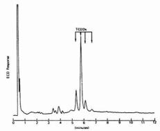
Figure 5. Temperature-programmed GC-ECD chromatogram for caustic extracted 2,3,6-TCP pyrolyzate, conditions in text.
