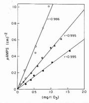
Figure 7. Current sensitivities at 13 °C ( $\bullet$ ), 22 °C ( $\bullet$ ), and 32 °C (O) at +0.6 V (vs. SCE)
