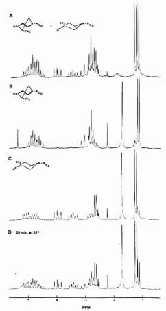
Figure 3. 100-MHz <sup>1</sup>H NMR spectra of *N*-nitroso-3 methyl-4-piperidone at -20 °C in CDCl<sub>3</sub>. (A) Equilibrium mixture of two isomers. (B) Low  $R_1$  isomer isolated by cryogenic TLC. (C) High  $R_1$  isomer isolated by cryogenic TLC. (D) Same sample as C, after warming to 22 °C for 20 min. Impurity peaks at  $\delta=1.8,\,2.1,\,$  and 5.3 are water, acetone, and methylene chloride, respectively
