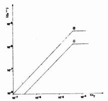
**Figure 4.** Cupric ion concentration as a function of total added copper concentration—malachite precipitation. (1)  $C_{\rm T}=2.65\times 10^{-3}$  M, pH 7.88; (2)  $C_{\rm T}=2.49\times 10^{-3}$  M, pH 7.70
