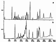
Figure 2. Reconstructed gas chromatograms for (a) 100 μg/L pure standard mixture and (b) 100 μg/L standard mixture containing soap when foam was allowed to enter the sorbent trap
