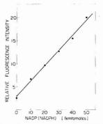
Figure 5. Analytical curve for the quantitation of NADP (NADPH) by enzyme amplification laser fluorimetry. The cycling volume is 100  $\mu$ L. The detection limit is 10 fmol (0.1 nM)
