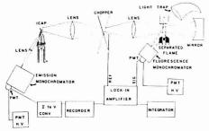
Figure 1. Diagram of experimental layout of components for measurement of ICAP-excited AFS and ICAP emission
