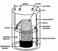
Figure 1. Cold/continuous development apparatus
