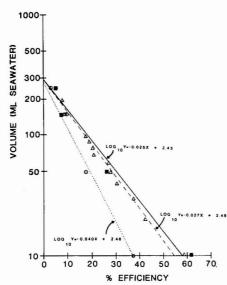
Figure 8. Adsorption of benzene from 50 ( $\odot$ ...), 100 ( $\triangle$ ---), 150 ppm ( $\blacksquare$ ---) seawater solutions by Sep-Pak C<sub>18</sub> cartridges as a function of sampling volume
