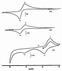
Figure 3. Fate of oxidized apomorphine at pH 4.5. Cyclic voltammograms were taken: (a) Before electrolysis, 4.37 mg apomorphine-HCl in 10 mL 1.2 M HCl. (b) After 2 e<sup>-</sup> electrolysis, oxidized apomorphine in 1.2 M HCl. (c) Immediately after adequate amount of buffer was added to allow the pH to reach 4.5. 1:1 ratio of apomorphine:oxoapomorphine
