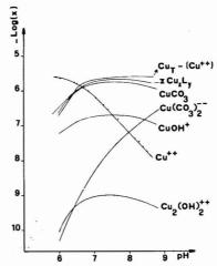
**Figure 5.** Copper carbonate and hydroxo complex distribution as a pH function.  $Cu_T=2.50\times 10^{-8}$  M;  $C_T=2.62\times 10^{-3}$  M (NaHCO<sub>3</sub>);  $L=OH^-$  or  $CO_3^{2-}$ ; x=1 or 2; y=1 or 2
