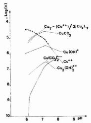
**Figure 6.** Copper carbonate and hydroxo complex distribution as a pH function.  $Cu_T=3.88\times 10^{-5}$  M;  $C_T=2.62\times 10^{-3}$  M (NaHCO<sub>3</sub>);  $L=OH^-$  or  $CO_3^{2-}$ ; x=1 or 2; y=1 or 2
