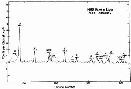
Figure 6. Prompt  $\gamma$ -ray spectrum of NBS Bovine Liver (SRM 1577) in the region of 3000 to 3450 keV. Note that this portion of the spectrum was taken at the same time as that of Figure 5, but the channel number scale is not the same because of the use of a biased amplifier for this and Figure 7. (See caption of Figure 3)
