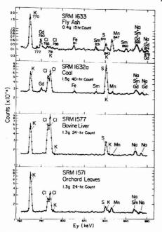
Figure 8. Expanded plots of the prompt  $\gamma$ -ray spectra of NBS standards in the vicinity of the 841-keV S line
