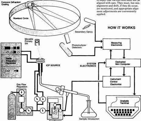
Figure 6. Schematic diagram of an ICP polychromator
