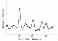
Figure 6. Example of correlation noise due to PRBS cycle length. Column was a 50-cm long, 2-mm l.d. copper tubing packed with 100/120 mesh Porapak P. Solute = acetone at 120 °C. k'=2.5. Other parameters were the same as in Figure 2, except for  $\pm 20\%$  modulation.
