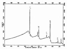
Figure 1. Widescan ESCA spectrum of the unused catalyst number 317 (Ketjen). The major primary peaks are noted
