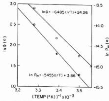
Figure 8. In  $\phi$  (O) vs. 1/T (K)  $\times$   $10^{-3}$ , In Pm (O) vs. 1/T (K)  $\times$   $10^{-3}$ at 13, 22, and 32 °C
