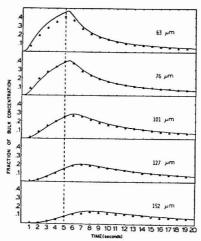
Figure 5. Fractional concentration vs. time at various distances for a double-potential step experiment. Numbers indicate distances from electrode. Solid lines are theoretical, points are experimental. Step from -0.20 to +0.20 V vs. SCE at t=0.0 s. Step from +0.20 to -0.20 V vs. SCE at t=5.0 s.
