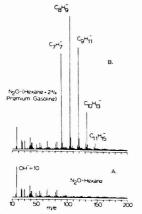
Figure 1. OH<sup>-</sup> spectrum of hexane (A) and a 2% solution of a gasoline in hexane (B)
