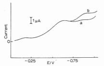
Figure 4. Linear potential scan voltammetry of nitrite at vitreous graphite in the catalytic medium. Conditions the same as in Figure 1b and 1c for a and b, respectively. Curves a and b superimpose in region not shown
