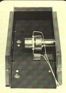
Refraction index free 8 µl flow through cell for applications in the liquid chromatography field.
