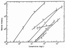
Figure 4. Composite of working curves. Bars on each line indicate the upper and lower limits of the normal clinical concentration range. (a) Ascorbic acid, (b) uric acid, (c) creatinine, (d) glutathione, (e) glucuronic acid, (f) glucose, (g) lactose
