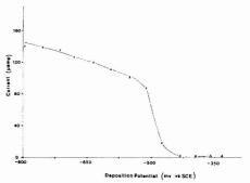
Figure 4. Pseudopolarogram of lead species in geothermal water
