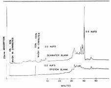
Figure 1. Comparison of liquid chromatographic system blank and trace enrichment chromatogram of 250 mL of uncontaminated seawater
