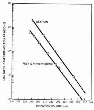
Figure 4. Calibration curves for poly(2-vinylpyridine) and dextran in 0.1 N HNO<sub>3</sub> + 0.1 N NaNO<sub>3</sub> on a 10-column set of quaternized supports varying in porosity from 40 to 25 000 Å. Flow rate = 2 mL/min
