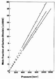
Figure 2. Partition isotherms for carbon dioxide in n-hexadecane at 25, 40, and 50 °C. Literature data at 760 Torr is the same as Figure
