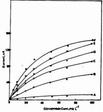
Figure 6. Glycoprotein calibrations at various pH values in the DPP mode at  $60 \text{ S h}^{-1}$  with TiO<sup>2+</sup> reagent concentrations at  $5.0 \times 10^{-2} \text{ M}$ : (A) pH 3.48, (B) 2.25, (C) 1.99, (D) 1.83, (E) 1.73, (F) 1.67
