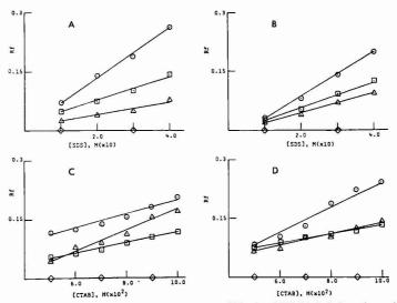
Figure 2. Plots of  $B_i$  value vs. surfactant concentration for DDE (Θ), DDT (Ξ), DDD (Δ), and DCB (♦). In A, the stationary phase is polyamide and the surfactant is SDS. In B, the stationary phase is alumina and the surfactant is SDS. In C, the stationary phase is polyamide and the surfactant is CTAB. In D, the stationary phase is alumina and the surfactant is CTAB.
