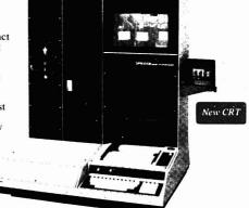
SP 8000B high-performance liquid chromatograph includes CRT, alphanumeric keyboard and printer/plotter for combined chromatogram and data reports.
