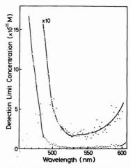
Figure 6. Detection limit of riboflavin (pH 6-7). Excitation source: PBD dye laser (377 nm)
