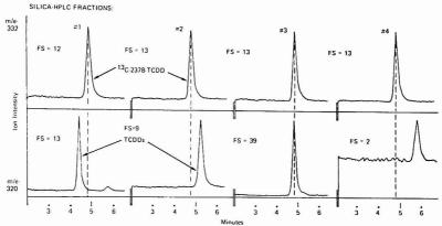
Figure 9. Composite mass chromatograms for silica-HPLC TCDD fractions #1 through #4, conditions in text. Ion m/e<sup>-</sup> = 332 is <sup>13</sup>C-2,3,7,8-TCDD retention time marker
