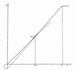
**Figure 1.** Typical enthalpogram obtained during neutralization of a glutaric acid solution ( $C_{\rm A}$  = 115  $10^{-4}$  mol L<sup>-1</sup>,  $V_{\rm 0}$  =  $10^{-1}$  L) by a sodium hydroxide solution ( $C_{\rm B}$  = 1.91 mol L<sup>-1</sup>)
