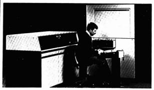
PW 1600/10 is a microprocessor-controlled simultaneous X-ray fluorescence spectrometer. It provides fixed channel simultaneous measurement of up to 28 elements, while scanning channels allow the identification and measurement of nonroutine elements. It can be used either as a stand-alone system or as an integrated element in an automatic process control analysis line. A universal interface allows for connection to any type of mini- or mainframe computer. Phillips
