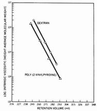
Figure 5. Log (hydrodynamic volume) vs. retention volume for poly-(2-vinylpyridine) and dextran in 0.1 N HNO $_3$  + 0.1 N NaNO $_3$  on a 10-column set of quaternized supports varying in porosity from 40 to 25 000 Å. Flow rate = 2 mL/min
