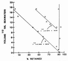
Figure 6. Adsorption and retention of toluene from seawater by Sep-Pak  $C_{10}$  cartridges as a function of pre-  $(\Delta)$  and post-sampling rinses (O) (constant 10-mL sampling volume) and variable sampling volumes ( $\square$ ), (no rinses)
