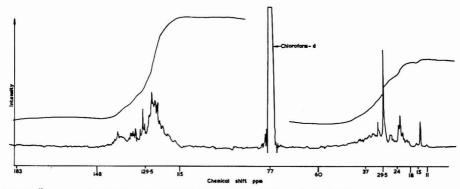
Figure 4. 13C spectrum of residue from a product oil of hydrogenated supercritical gas extract (extract d)
