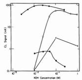
Figure 3. Variation of CL signal with KOH concentration. Lophine =  $3.2\times10^{-4}$  M;  $H_2O_2=1.0\times10^{-3}$  M. OCI ( $\bullet$ ), Cu(II) (O), Cr(III) ( $\blacksquare$ ) Co(II) ( $\Box$ ), VO<sup>2+</sup> (X)
