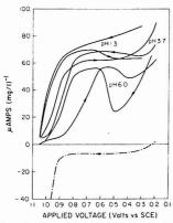
Figure 4. Current-voltage relationship at the rotating gold electrode in 0.05 M  $_{\rm H_2}$ SO<sub>4</sub> (pH 1.3), 0.5 M  $_{\rm K_2}$ SO<sub>4</sub> (pH 3.7), and 0.5 M  $_{\rm K_2}$ SO<sub>4</sub> (pH 6.0). Solid lines are for ozone reduction current and dashed lines are residual current
