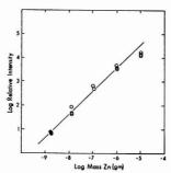
Figure 5. Analytical curve for Zn in powder samples with a graphite
