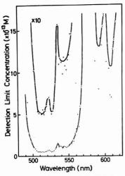
Figure 4. Detection limit of fluorescein (pH 13). Excitation source: esculin dye laser (480 nm)
