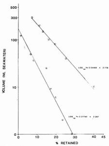
Figure 7. Adsorption of benzene from seawater by Sep-Pak C<sub>18</sub> cartridges as a function of post-sampling rinses, ⊙ (constant 10-mL sampling volume) and variable sampling volumes, □ (no rinses)
