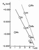
Figure 2. Plot of  $R_{M_{COT}}$  from  ${\rm Hg^{2+}}/{\rm chloroform}$  system vs. number of carbon atoms in alkyl R in Ph-S-R (I-V, VII)
