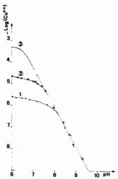
**Figure 1.** Cupric ion concentration (log) as a pH function (carbonate free solutions). (1) Cu<sub>T</sub> =  $1.55 \times 10^{-6}$  M; (2) Cu<sub>T</sub> =  $3.88 \times 10^{-5}$  M; (3) Cu<sub>T</sub> =  $9.95 \times 10^{-4}$  M
