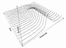
Figure 2. Sequence of runs used to generate pseudopolarogram
