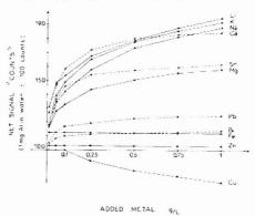
Figure 3. Action of different metals on 1 mg/L Al signal intensity
