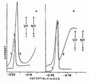
Figure 3. Comparison of performances of (1) hanging mercury drop electrode and (2) mercury-coated glassy carbon electrode for (a) compound I and (b) compound II. Concentrations are (1a)  $3 \times 10^{-6}$  M; (2a)  $6 \times 10^{-3}$  M; (1b)  $2 \times 10^{-5}$  M; (2b)  $10^{-6}$  M in 0.05 M KNO<sub>2</sub>/HNO<sub>3</sub>. Current ranges as shown
