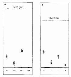
Figure 1. Tracing of developed chromatograms. Chromatogram A consists of a polyamide stationary phase developed with a 4.0 × 10<sup>-1</sup> M SDS<sub>ag</sub> solution. Chromatogram B shows the separation of uridine (U), guanosine (G), cytidine (C), and adenosine (A) using reverse phase TLC. The mobile phase consisted of 1.5 M sodium dioctylsulfosuccinate and 4.44 M H<sub>2</sub>O in cyclohexane
