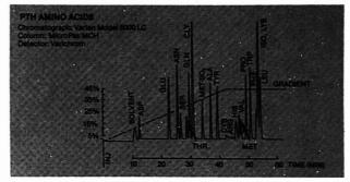
Twenty PTH amino acids can be separated in a single gradient run on the Varian Model 5000 Liquid Chromatograph. For more information circle Reader Service Number 235.
