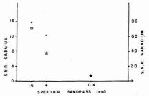
Figure 2. Effect of spectral bandpass on the ICAP-excited AFS signal-to-noise ratio from ( $\blacksquare$ ) cadmium in a nitrogen-separated air/acetylene flame and ( $\dot{x}$ ) vanadium in a nitrogen-separated nitrous oxide/acetylene flame (20 ng/mL Cd; 100  $\mu$ g/mL V)
