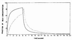
Figure 8. Fraction of bulk concentration vs. time for 13 µm from electrode surface. Double-step experiment. Solid line, theoretical; dashed line, experimental.
