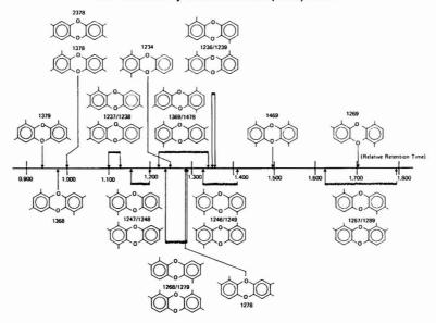
Figure 11. TCDD isomer elution sequence for silica-HPLC, approximate 2,3,7,8-TCDD absolute retention time is 14.70 min and is defined as 1.000; refer to text for description
