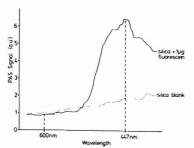
Figure 1. Spectrum of fluorescein on a silica gel-coated aluminumbacked TLC plate
