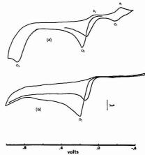
Figure 4. Interaction of oxidized apomorphine with glutathione. Apomorphine  $\sim 1\times 10^{-3}$  M in pH 7.4 phosphate buffer, scan rate 3 V/min. Glutathione concentrations: (a)  $1.0\times 10^{-3}$  M; (b)  $5.0\times 10^{-3}$  M
