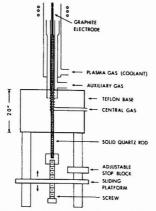
Figure 1. Schematic drawing of the direct sample insertion torch
