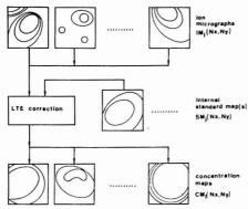
Figure 1. Quantitative image correction, using LTE algorithm (schematic)
