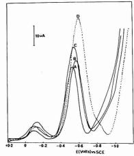
**Figure 2.** Continuous-flow differential pulse scans of the reagent, potassium titanium oxalate ( $5.0 \times 10^{-2}$  M) with varying glycoprotein concentrations. (A) 0, (B) 20, (C) 100, (D) 300 mg L<sup>-1</sup>
