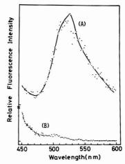
Figure 2. Fluorescence spectrum of riboflavin (pH 6–7), 1  $\times$  10<sup>-9</sup> M) (A) and background spectrum of solvent water (B). The Raman band of water is located at 431 nm (not shown). Excitation source: PBD dye laser  $(\lambda_{ss}=377 \text{ nm}, \Delta\lambda_{ss}=0.4 \text{ nm})$
