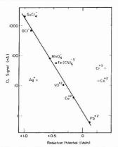
Figure 1. Correlation of the CL signal and the reduction potential of the analyte. The line is the least-squares fit to the solid data points
