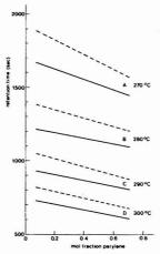
Figure 7. Retention time vs. mole fraction perylene in a mixture of 3,4-benzopyrene and perylene. Mole fraction 0.2 means 0.2 × 500 = 100 ng perylene and 400 ng 3,4-benzopyrene per µL benzene. The dotted line is the retention behavior of 3,4-benzopyrene
