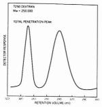
Figure 2. Chromatogram of a 250 000 mol wt dextran in 0.1 N HNO<sub>3</sub> + 0.1 N NaNO<sub>3</sub> on an 8-column set of quaternized supports varying in porosity from 170 to 25 000 Å. Flow rate = 2 mL/min
