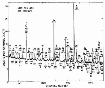
Figure 2. Prompt  $\gamma$ -ray spectrum of NBS Fly Ash (SRM 1633a) in the region of 515 to 890 keV
