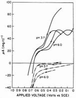
Figure 3. Current-voltage relationship at the rotating gold electrode in 1.6 M KCl (pH 6.0) and 0.5 M KCl (pH 9.7). Solid lines are for ozone reduction current and dashed lines are residual current
