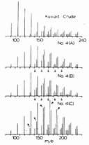
Figure 4. OH<sup>-</sup> spectrum of a Light Kuwait Crude, as uncontaminated (A) and contaminated (B) sample of a No. 4 Fuel Oil, and an uncontaminated No. 4 Fuel Oil from a different manufacturer (C). See text for meaning of the open and darkened circles
