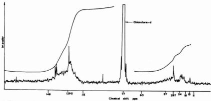
Figure 3. <sup>13</sup>C spectrum of aromatic fraction of the *n*-pentane solubles from a supercritical gas extract prepared in the presence of hydrogen and catalyst (extract c)
