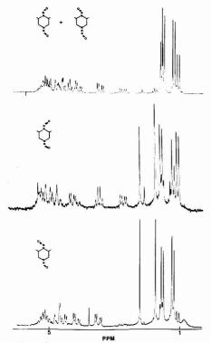
Figure 4. 100-MHz <sup>1</sup>H NMR spectra of dinitroso-2,6-dimethylpiperazine. (A) Equilibrium mixture at 25° C. (B) High R, isomer at -40 °C, isolated by cryogenic TLC. Impurity peaks are acetone at  $\delta = 2.1$ , water  $\delta$ = 1.8, and diethyl ether (developing solvent) at  $\delta$  = 3.4 and 1.2. (C) Low R, Isomer at -40 °C, isolated by cryogenic TLC. Impurity peaks are acetone at  $\delta = 2.1$  and water at  $\delta = 1.8$
