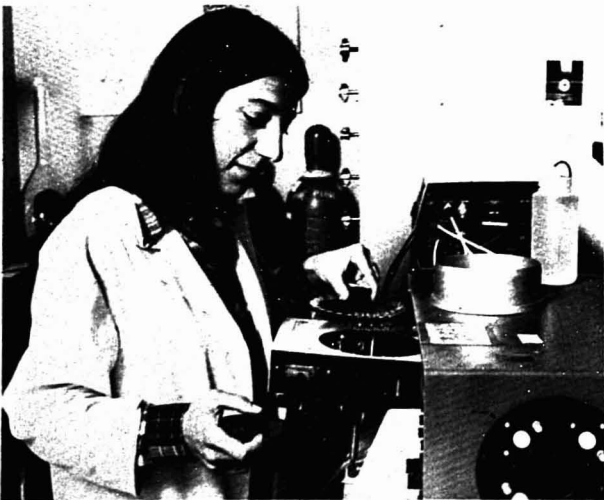
Barbara Ehrlich is putting blood serum samples into the spectrometer's automatic sampler in preparation for lithium analysis
