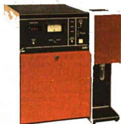
Model 3010 Trace Metals Analyzer. Measures up to 200 micro or macro samples daily at 90 seconds or less per sample using a rapid exchange reagent. Cost per sample: about one-third that of conventional methods. Excellent accuracy and precision at the nanogram level. Circle No. 65
