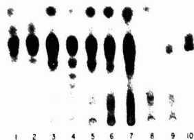
Figure 4. TLC plate of oligo- and polysaccharide fractions from honey, honey-HFCS mixtures, HFCS and standard trisaccharides
