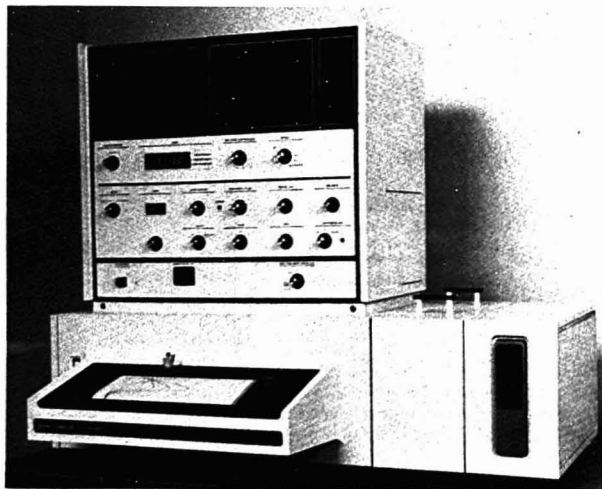
The Cary 210 UV-VIS spectrophotometer has an absorbance range of -0.6000 to +4.000. The electronic-based baseline corrector is programmable for different scan conditions. Operating parameters such as scan speeds, slit widths, and absorbance ranges are varied using the front panel. The roomy sample compartment can accommodate two five-cell turrets, microcells, and cylindrical cells. Price is $11 995. Varian Instrument Division 406
