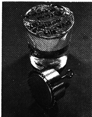
Figure 3. Rod holder for dip coating with beaker of polymer solution
