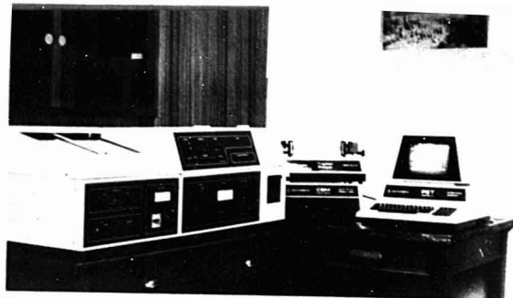
Figure 7. Photoacoustic spectrometer pictured with a Commodore PET computer, floppy disc drive, and printer. The spectrometer is manufactured by EDT Research, 14 Trading Estate Rd., Great Western Trading Estate, Park Royal, London NW10 7LW, England.
