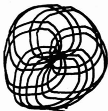
Figure 1. Pattern traced by arm of Minimet Polisher/Grinder.
