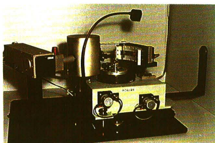
STOE transmission goniometer with curved focusing monochromator.
