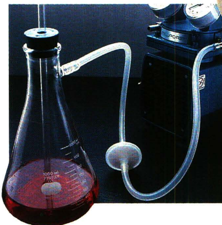
Right—The Millex-FG 50 unit has many laboratory applications, including the protection of pumps and vacuum sources from damage by liquid aerosols.
