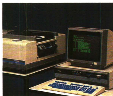
Nicolet low-cost 5DXC FT-IR with Autosampler analyzes up to eighty QC samples automatically.
