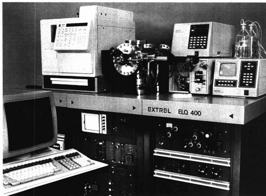
ThermoBeam LC/MS is a particle beam-type interface that removes LC solvent from analytes before they enter the mass spectrometer. Various LC separation conditions or MS ionization modes are possible. Extrel 401
