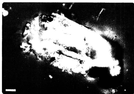
Figure 3. Same parchment fragment in Figure 2 shown here with slightly uncrossed polars. The small white particles are calcite (limestone); the smaller dark particles are anatase. This is a transmitted light micrograph with slightly uncrossed polars. The bar represents 20 \mu m.
