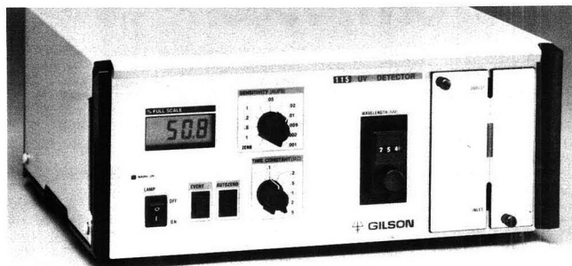
Model 115 variable-wavelength UV detector features a sensitivity range of 0.001–1.0 AUFS (10-mm light path), 2% typical peak-to-peak noise levels at 0.001 AUFS, and front-panel wavelength, sensitivity, and time constant controls. Gilson Medical Electronics 401
