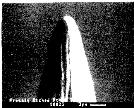
Figure 1. Scanning electron micrograph (SEM) of the tip of a Pt-Ir wire after electrochemical etching.
