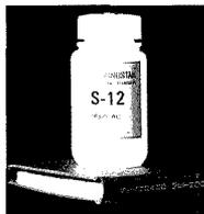
The metal content in each Canostan oil-based calibration standard is determined by chemical assay methods with results that are traceable to NIST standards (where applicable). This traceability means Canostan
