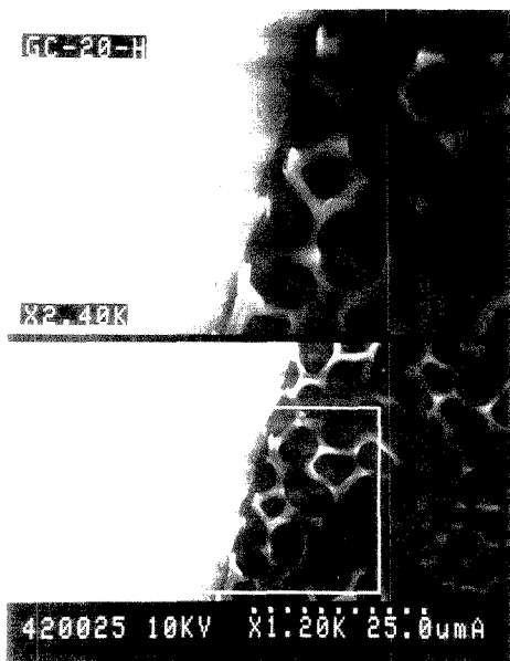
Figure 1. SEM photomicrograph of a spin-coated poly(4-vinylpyridine) film that has been cross-linked using 1,6-dibromohexane. The magnification is 2.4k (upper) and 1.2k (lower), respectively. The film has been mechanically removed from the glassy carbon surface on the left half of the photograph.
