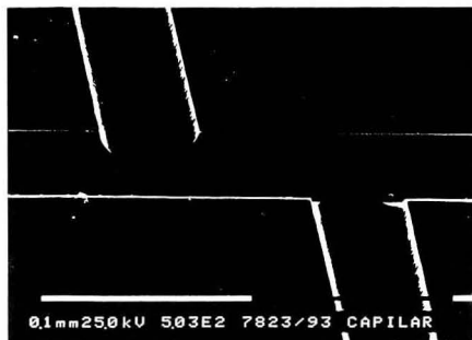
Figure 2. Electron micrograph displaying details of the injection volume. The horizontal capillary represents the separation channel; the vertical channels in the left and right parts of the micrograph are connected to reservoirs 1 and 4, respectively. The distance between the outside walls of the injection channels defining the plug length is 150 \mu\text{m} .
