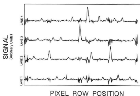
Figure 6. One-dimensional representation of lanes with selective accumulation as prescribed by the expert system. Peaks are smaller in rows with fewer frames of data accumulated, but S/N is constant for each recognized feature in the image.
