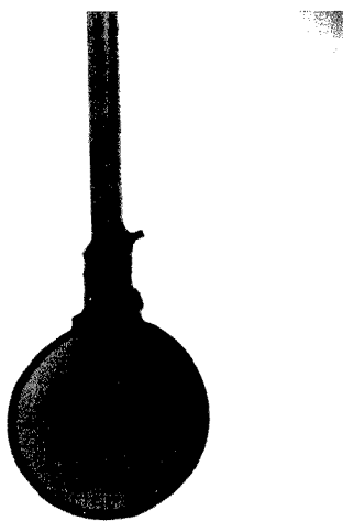
Figure 4. Photomicrograph of the liquid film formed on the loop. A thin film was made with an aqueous solution of 2.6 mM Malachite Green for easier visualization. The scale is indicated by the diameter of the wire, 100 \mu\text{m} .
