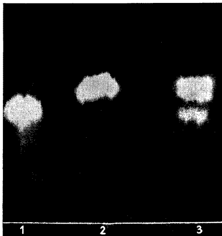
Fig. 4. Resolution of tryptophan isomers on paper chromatography. Whatman No. 1 filter paper was developed with methanol-water solvent (9 : 1) for 48 h, dried and examined as described in text. 1. l -tryptophan; 2. d -tryptophan; 3. dl -tryptophan.
