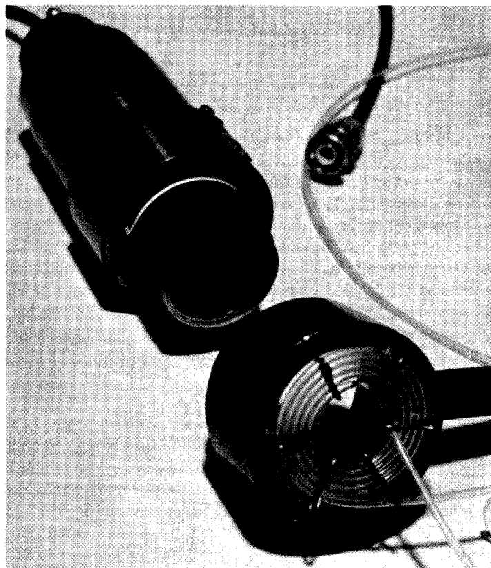
Fig. 1. Photograph of flow monitor, disassembled to show both the GM tube holder and the spiral arrangement.
