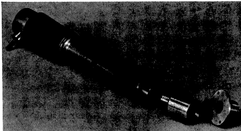
Fig. 3. Electrode assembly used in absorption tube.
