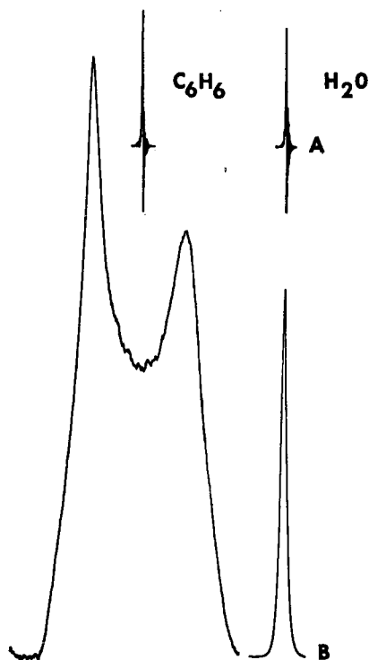
Fig. 4. Bulk susceptibility determination with 3-mm inner tube cell. Spectra A: spinning system; spectra B: static system.
