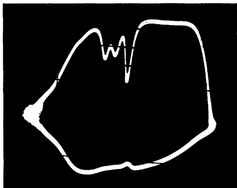
Fig. 3. Supporting electrolyte with 2 \cdot 10^{-5} M indium(III), 1.4 \cdot 10^{-5} M lead(II) and 2.5 \cdot 10^{-5} M cadmium(II).
