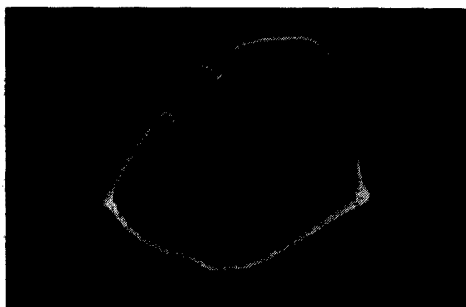
Fig. 2. Oscillopolarogram of supporting electrolyte D with 4 \cdot 10^{-5} M germanium(IV).
