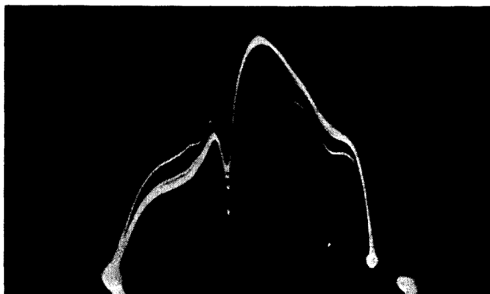
Fig. 9. dE/dt = f(E) curves for 1.5 \cdot 10^{-6} M Ni(II) in 0.5 M NH_4NO_3 - 0.25 M urotropine- 0.1 M NH_4SCN . Electrode polarized by several cycles of a.c.; during the quiescent period of 2.5 sec polarized at -0.4 V (the deepest incision corresponds to the first cycle).
