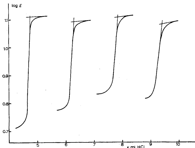
Fig. 1. Titration curves ( \log E (mV) against ml titrant added) for the titration of ca. 3, 4, 5 and 6 ml of Standard Sea Water with v ml of 0.02002 M hydrochloric acid. The curves have been corrected for basic impurities and indicator error.
