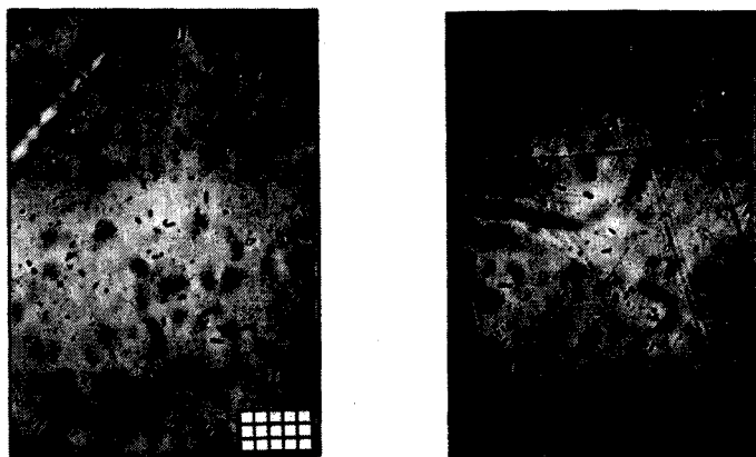
Fig. 3. Typical fission track patterns of condensed sea water samples. (a) Sample No. 2; (b) sample No. 3.
