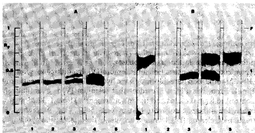
Fig. 2. Silica gel thin-layer chromatography. A = photograph, B = autoradiogram. (1) Mixture of elementary ^{75}\text{Se} and oxidation product of dithizone; (2) oxidation product of dithizone; (3) ^{75}\text{Se} dithizonate; (4) mixture of elementary ^{75}\text{Se} , ^{75}\text{Se} dithizonate and oxidation product of dithizone; (5) elementary ^{75}\text{Se} .
