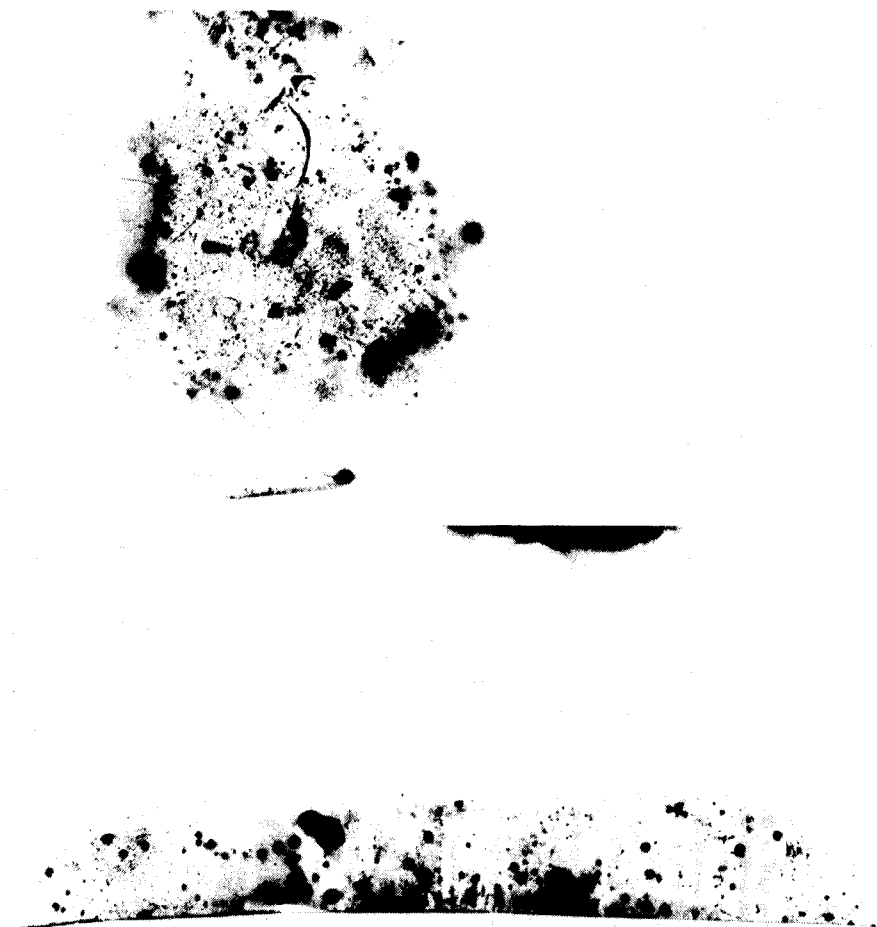
Fig. 3. Autoradiographs showing adsorption of chromium(III) on, above, beaker bottom, and, below, beaker sides.
