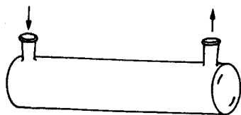
Fig. 2. Measuring cell with windows transparent to 253.7-nm radiation. Pathlength 1 cm and 10 cm.
